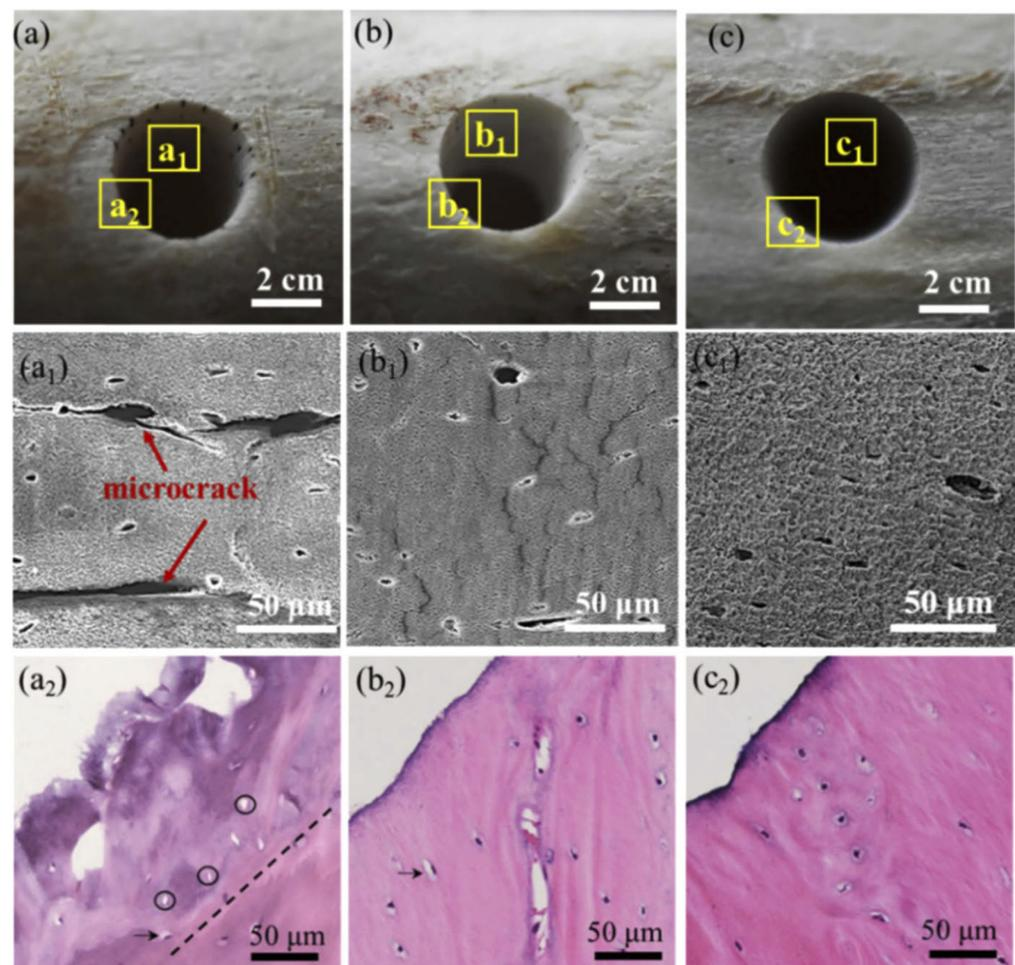
**Figure 2.** Morphology of laser-drilled bone tissues under different environmental cooling conditions. Vertical panels (a–c) correspond to without cooling, gas cooling and water cooling; horizontal panels (subscript: none, 1, 2) correspond to white light, SEM and histology images. Adapted from [42].
