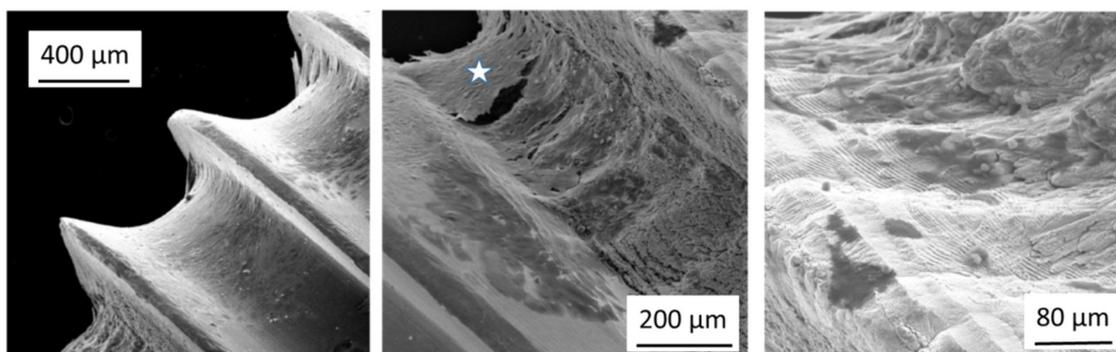
**Figure 3.** SEM image comparison of a pre-anodized titanium-based bone screw without femtosecond laser treatment (**left**) showing osteoblast growth and adhesion, and the same screw with femtosecond laser treatment (**middle**) showing cell-free areas, and details at higher magnification (**right**). Adapted from [86].
