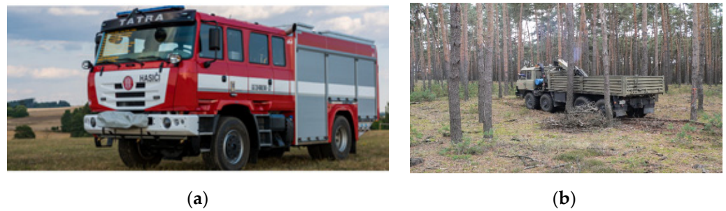
Figure 5. Fire and tested vehicles. (a) Fire vehicle Tatra 815 4 × 4, Length/Width/Height: 7950/2550/3000 mm. (b) Tested terrain vehicle Tatra 815 8 × 8, Length/Width/Height: 8950/2550/3300 mm.
