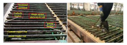
Figure 1. The nickel electrolytic cells and the conventional manual detection.
