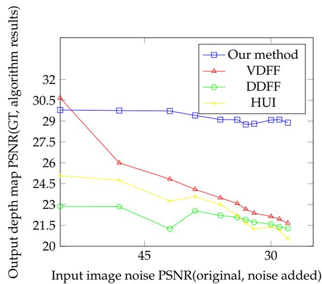
**Figure 15.** PSNR comparison adding camera simulated noise to input images. VDFF has better results in purely synthetic defocus without noise, but our approach is stable with different levels of noise.
