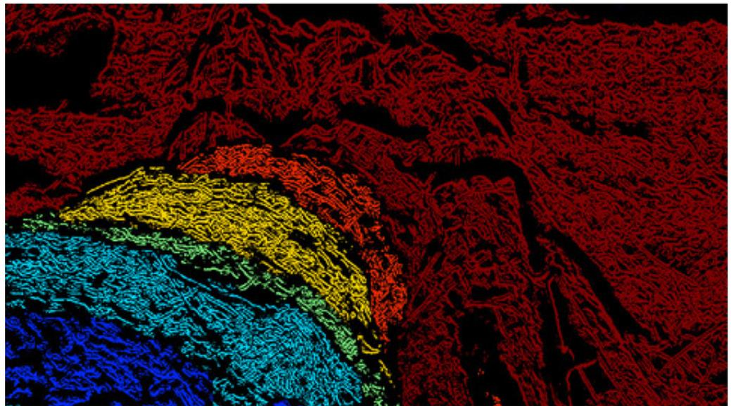
**Figure 5.** Sparse depth map represented in JET color space (blue-near, red-far), black means unknown information.
