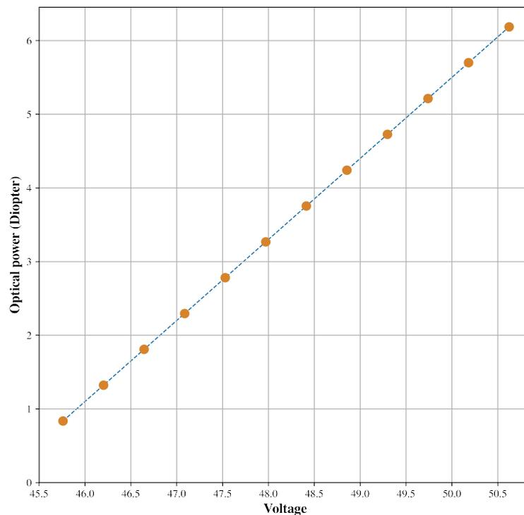
Figure 3. Chart displaying the  $V_{rms}$  values used with the lens and the correspondence optical power.
