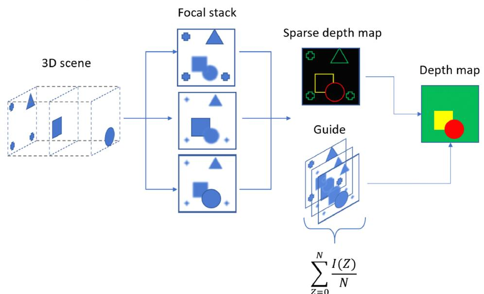
Figure 4. Algorithm pipeline.
