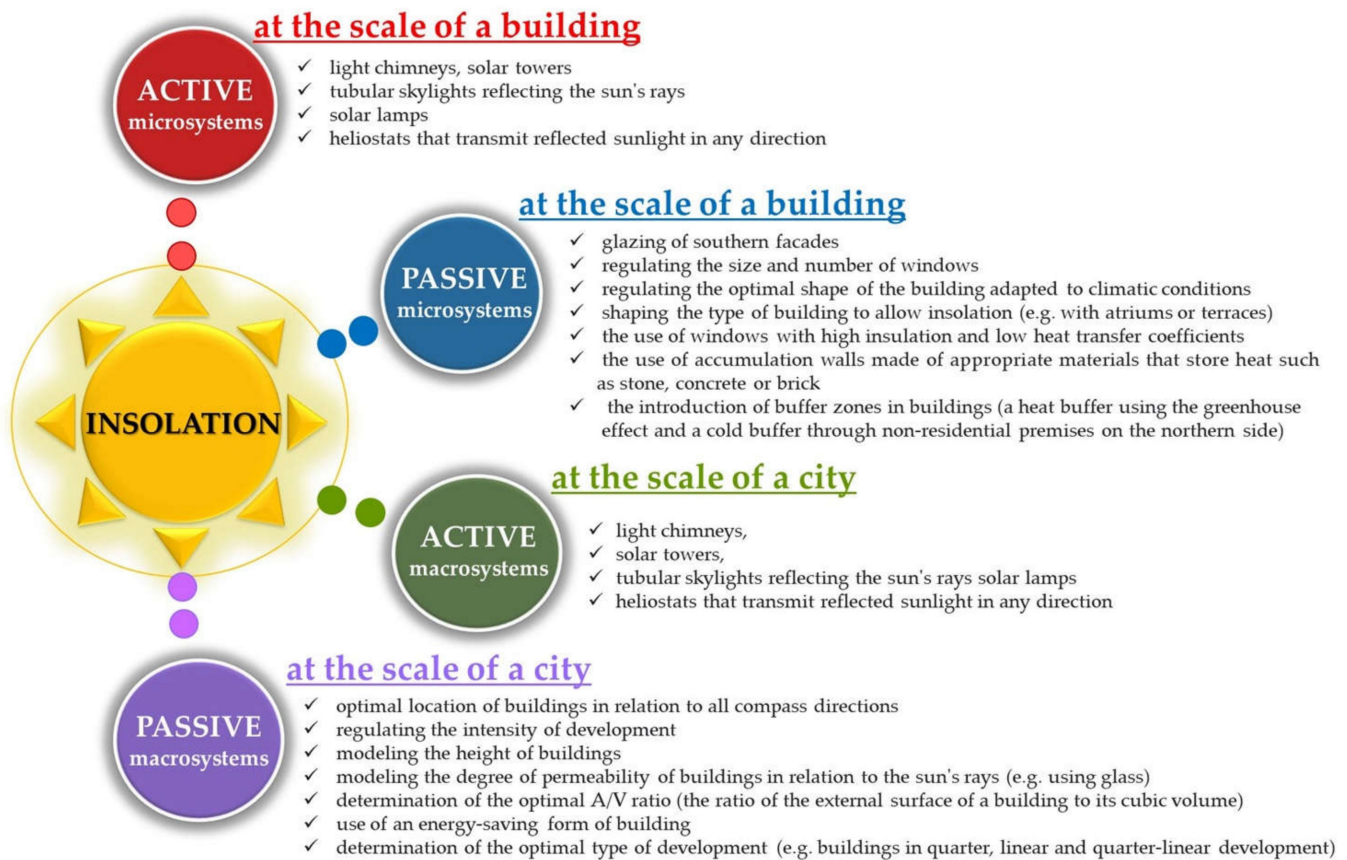
Figure 3. Multi-scale systems of passive and active insolation on micro- and macroscales (authors).
