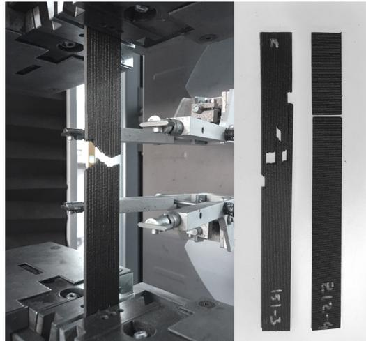
**Figure 2.** Tensile test setup with a tactile strain gauge and a fractured x-specimen with additional representation of fractured specimens for both the x- and z- direction of testing.
