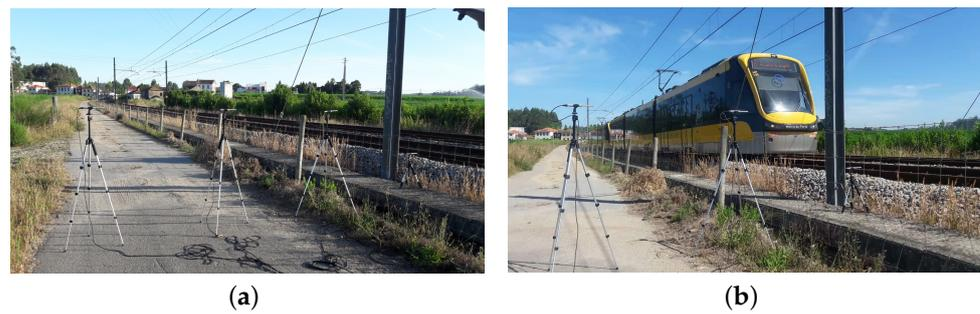
**Figure 4.** Photographs of the in situ experimental characterisation. (a) Photograph of the microphones on site. (b) Photograph of the measurement setup in the presence of the vehicle.
