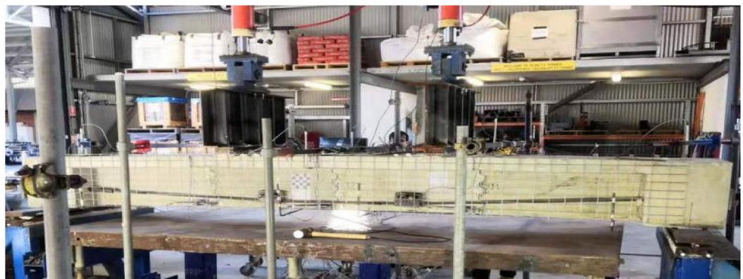
Figure 3. Tested precast prestressed concrete segmental beam.
