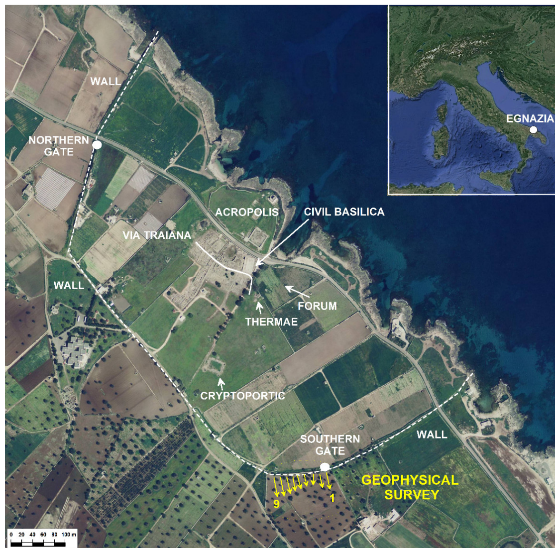
Figure 1. Survey plan on a 2008 TerraItaly™ Orthophoto with indication of the 1–9 parallel 2D Electrical Resistivity Tomography (ERT) lines (in yellow).
