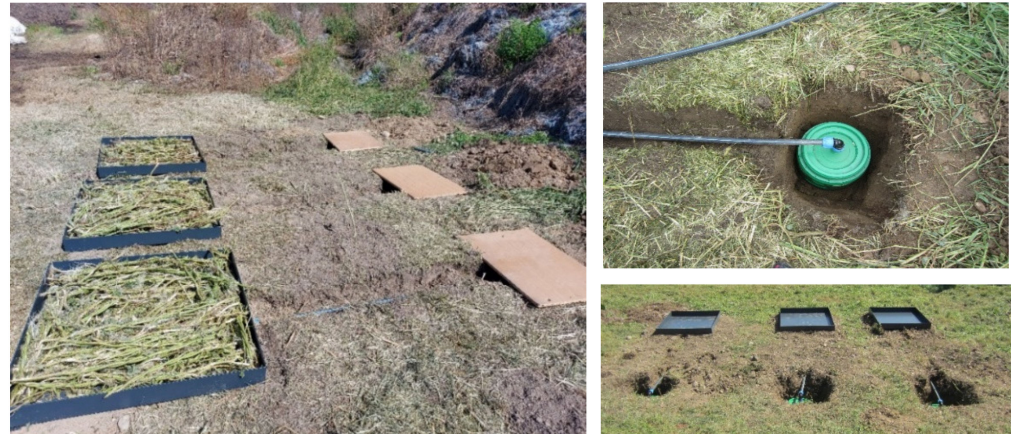
Figure 1. Metal drip tray setting.
