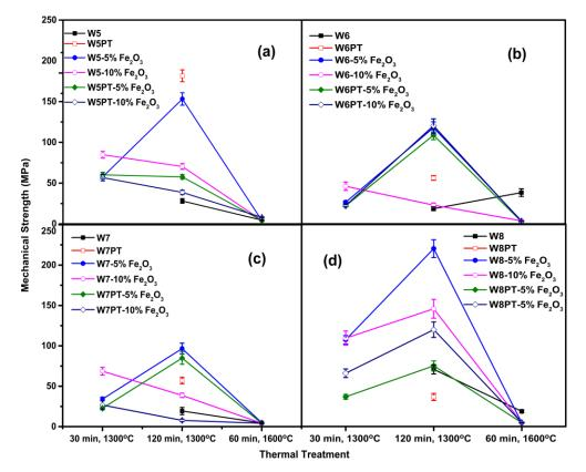
as of (undesirable) pyroxenes (consisting mainly of enstatite) decreases due to the binding of magnesium by hematite in the respective crystalline phases.
