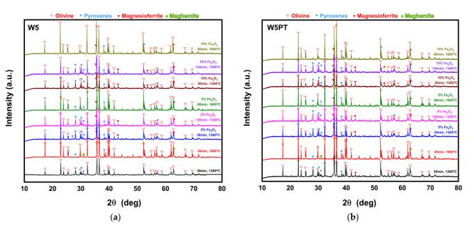
**Figure 7.** XRD patterns of the thermally treated products obtained from the respective samples: (a) W5, and (b) W5PT (with or without the presence of hematite).
