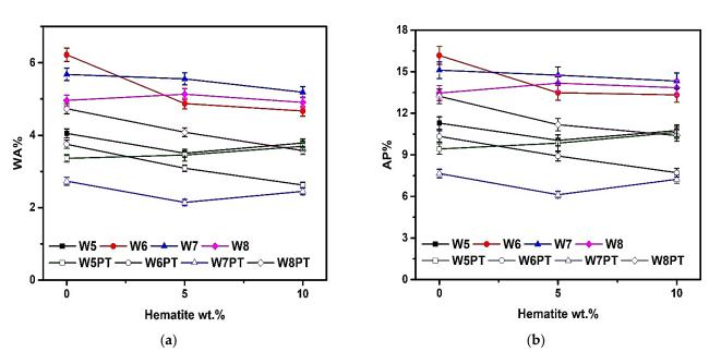
**Figure 4.** The effect of hematite addition on the values of (**a**) WA%, and (**b**) AP% parameters for the obtained products considering after the thermal treatment at 1300 °C for 30 min.
