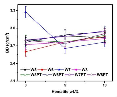
**Figure 5.** The effect of hematite addition (wt.%) on the BD ( $g/cm^3$ ) parameter for the examined samples after the thermal treatment at 1300 °C for 30 min.
