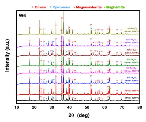
**Figure 8.** XRD patterns of thermally obtained products from sample W6 under different firing conditions with and without the addition of hematite.
