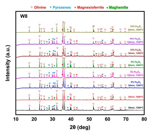
**Figure 10.** XRD patterns of the product obtained from the sample W8 under different firing conditions with and without the addition of hematite.
