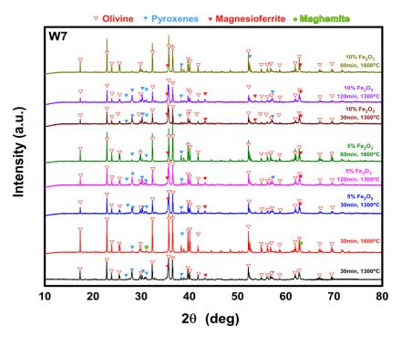
**Figure 9.** XRD patterns of thermally obtained product from sample W7 under different firing conditions with and without the addition of hematite.
