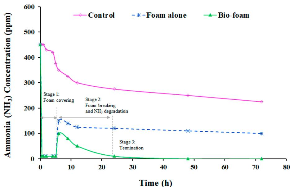
**Figure 4.** Change in  $\text{NH}_3$  concentration emitted from swine manure in the open reactor: control (no treatment, only manure), foam alone (application of surfactant foam only), and bio foam (surfactant foam containing bacteria). The initial  $\text{NH}_3$  concentration in the manure was 450 ppm.
