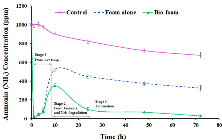
**Figure 3.** Change in  $\text{NH}_3$  concentration from  $\text{NH}_3$ -contaminated soil with time in the closed reactor; control (no treatment), foam alone (application of surfactant foam only), and bio-foam (surfactant foam containing bacteria).
