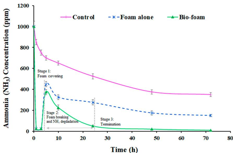
**Figure 2.** Change in  $\text{NH}_3$  concentration from  $\text{NH}_3$ -contaminated soil with time in the open reactor; control (no treatment), foam alone (application of surfactant foam only), and bio-foam (surfactant foam containing bacteria).
