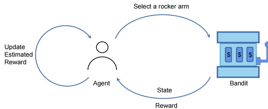
**Figure 2.** An illustration of the multi-armed bandit method. The agent can sense the state and obtain rewards by shaking the rocker arms. This process updates the estimated reward according to past rewards.
