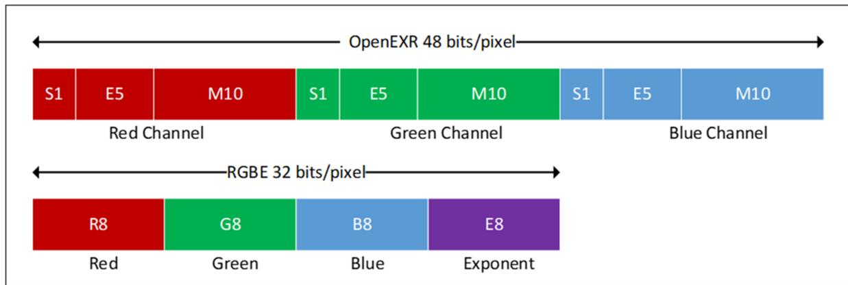
**Figure 2.** The bit breakdown for the 48-bit/pixel OpenEXR, 1-bit sign, 5-bit exponent, 10-bit mantissa, and 32-bit/pixel RGBE encodings, 8-bit in the Red, Green, Blue, and Exponent channel.
