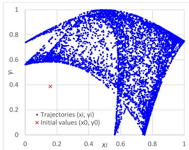
**Figure 3.** Trajectories of 2D-SLMM with an initial value  $(x_0, y_0) = (0.15874, 0.38797)$  and the control values  $(\alpha, \beta) = (1, 3)$ .
