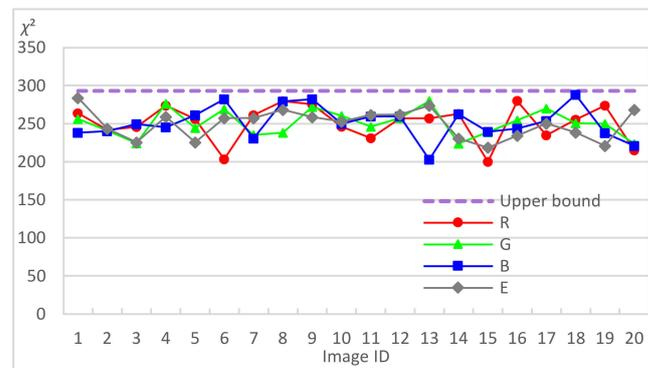
**Figure 8.** All 20 stego encrypted images in four channels pass the  $\chi^2$  test.
