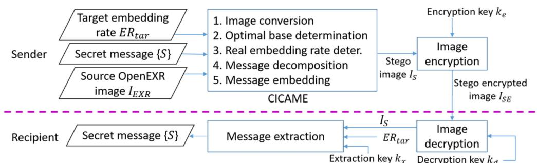
**Figure 1.** The flowchart of our proposed method consisting of message embedding and extraction processes.
