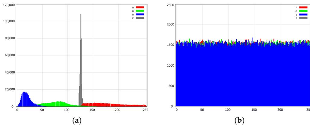
**Figure 7.** Histograms of the stego HDR RGBE image, “memorial”; (a) the histogram of the plain stego image; (b) the histogram of the stego encrypted image.
