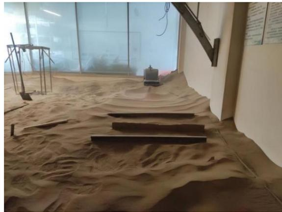
**Figure 8.** Laboratory experiment for preventing sand deposition on railway tracks.
