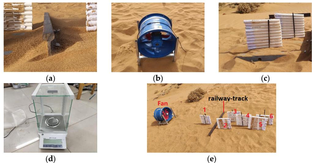
**Figure 2.** Sketches of the field experiment. (a) the track; (b) axial fan; (c) sediment collecting device; (d) electronic balances; (e) arrangement of experimental equipment.
