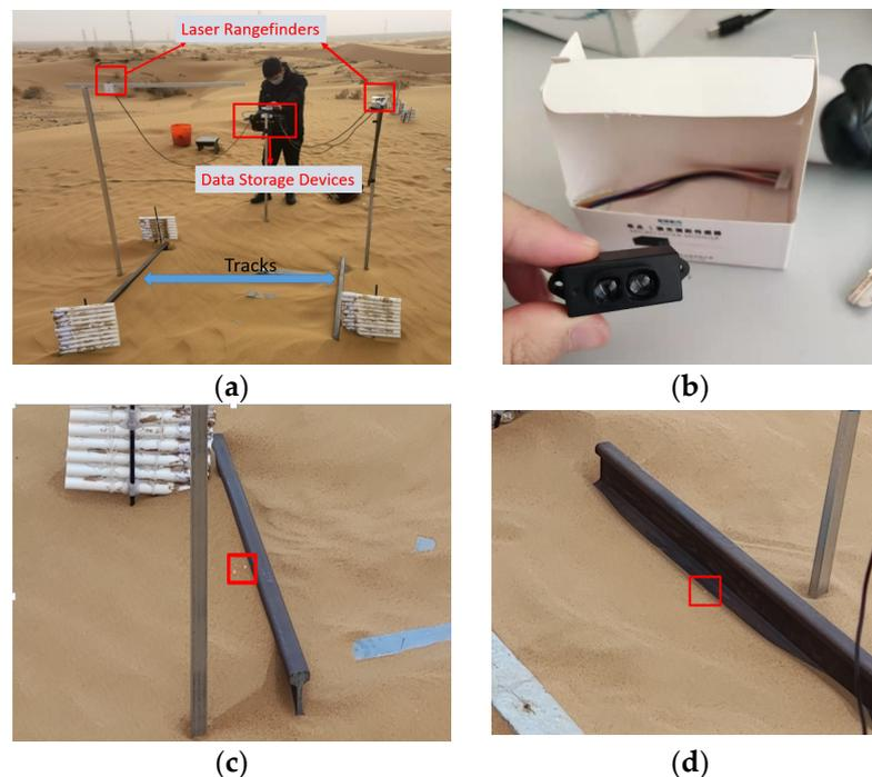
**Figure 5.** Scene of field experiment based on laser ranging. (a) field experiment; (b) laser rangefinders; (c) measurement point for the first track; (d) measurement point for the second track.
