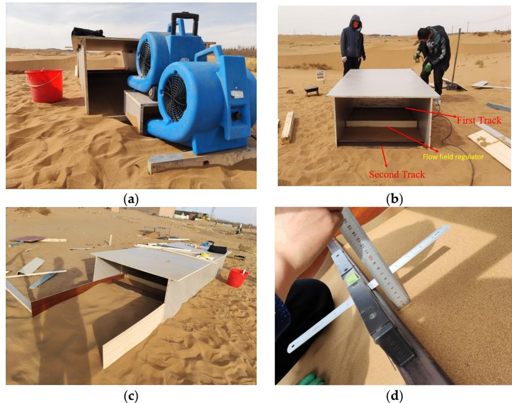
**Figure 7.** Schemes of Field Experiment Based on Simple Wind Tunnel. (a) simple experimental wind tunnel; (b) arrangement of the experimental devices; (c) general view of the experimental setup; (d) measurement of sediment height.
