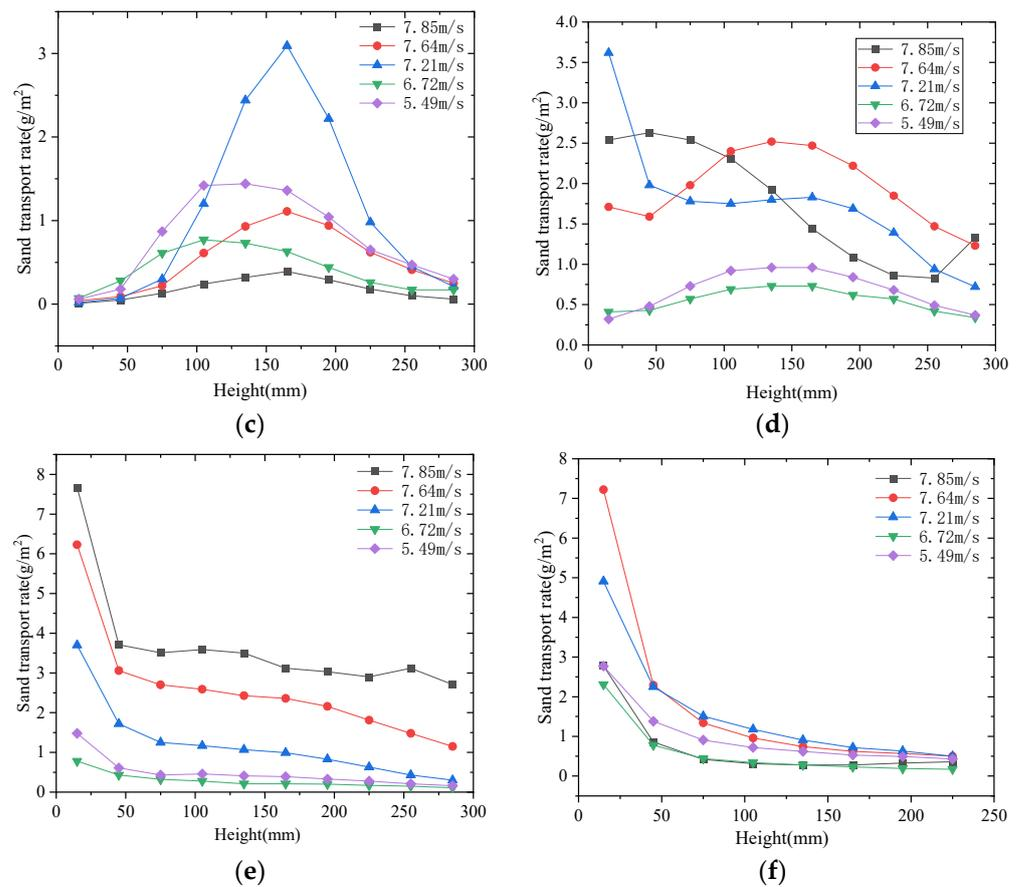
**Figure 3.** The sand transport rate of each sediment collecting device. (a) No. 1 sediment collecting device; (b) No. 2 sediment collecting device; (c) No. 3 sediment collecting device; (d) No. 4 sediment collecting device; (e) No. 5 sediment collecting device; (f) No. 6 sediment collecting device.
