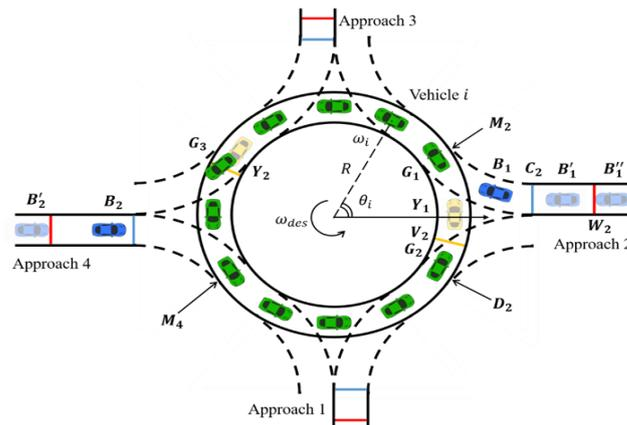
**Figure 3.** Illustration of self-adjusting stage and virtual platoon control stage in vehicles' merge-in procedure.
