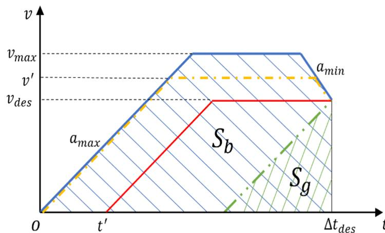
Figure 4. Feasible speed trajectories for vehicles in the self-adjusting stage.
