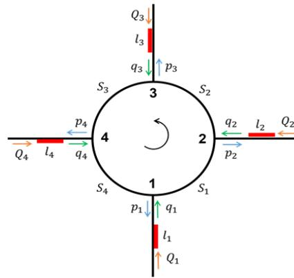
Figure 2. Four-approach roundabout.
