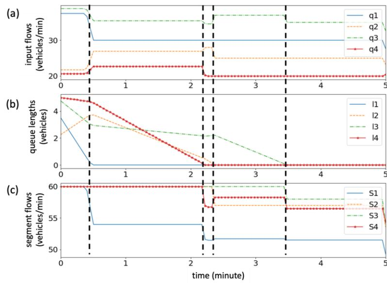
Figure 5. (a) Optimal merge-in flows; (b) queue lengths; (c) segment flows.
