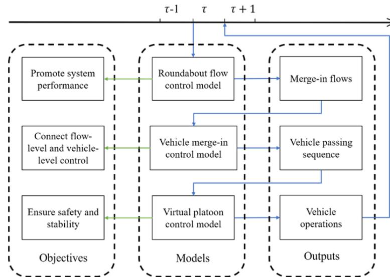
Figure 1. Conceptual structure of the roundabout control strategy.
