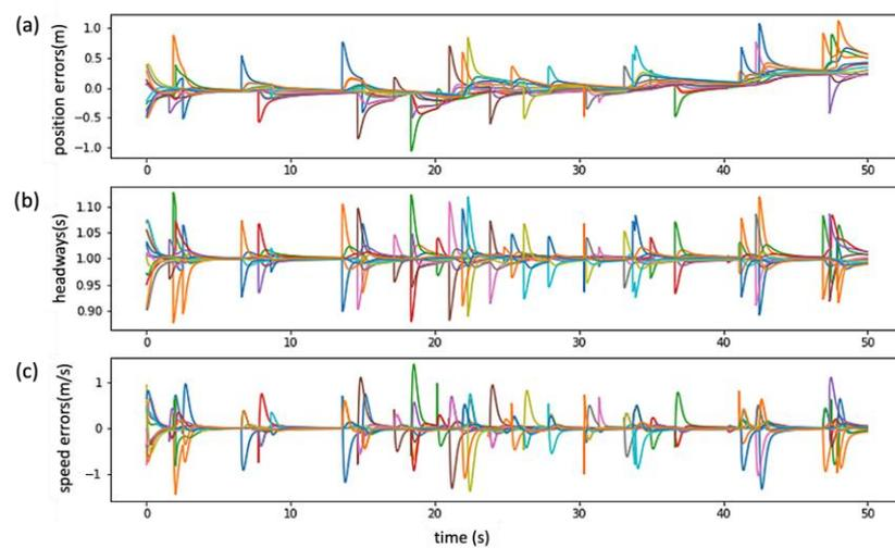
Figure 7. Stability and safety analysis of virtual platoon control: (a) position errors; (b) headways; (c) speed errors.
