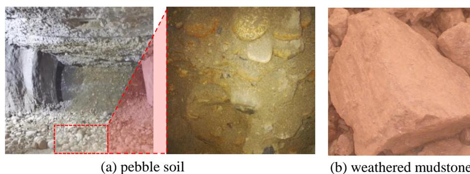
**Figure 4.** Soil layer of the tunnel excavation face.
