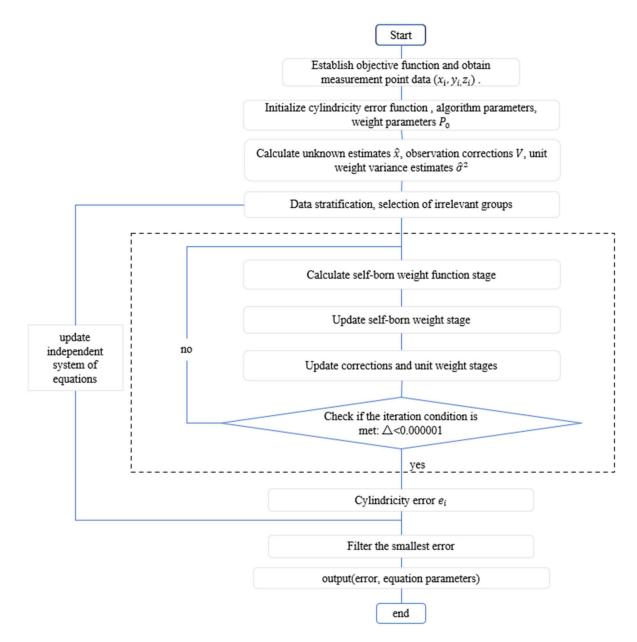
Figure 2. ISWLS cylindricity error algorithm evaluation process.
