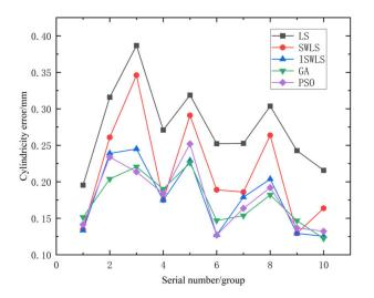
Figure 6. Cylindricity error evaluation comparison.
