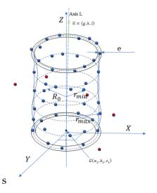
Figure 1. Diagram of cylindricity error.
