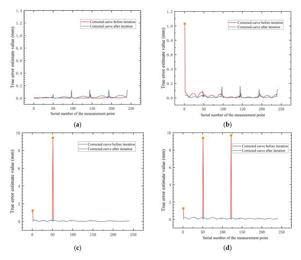
**Figure 7.** Statistics chart of true error value when inserting gross error points. (**a**) No gross error point insertion. (**b**) Insert one gross error point. (**c**) Insert two gross error points. (**d**) Insert three gross error points.
