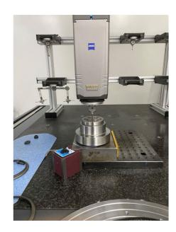
Figure 4. Cylindricity error measurement.
