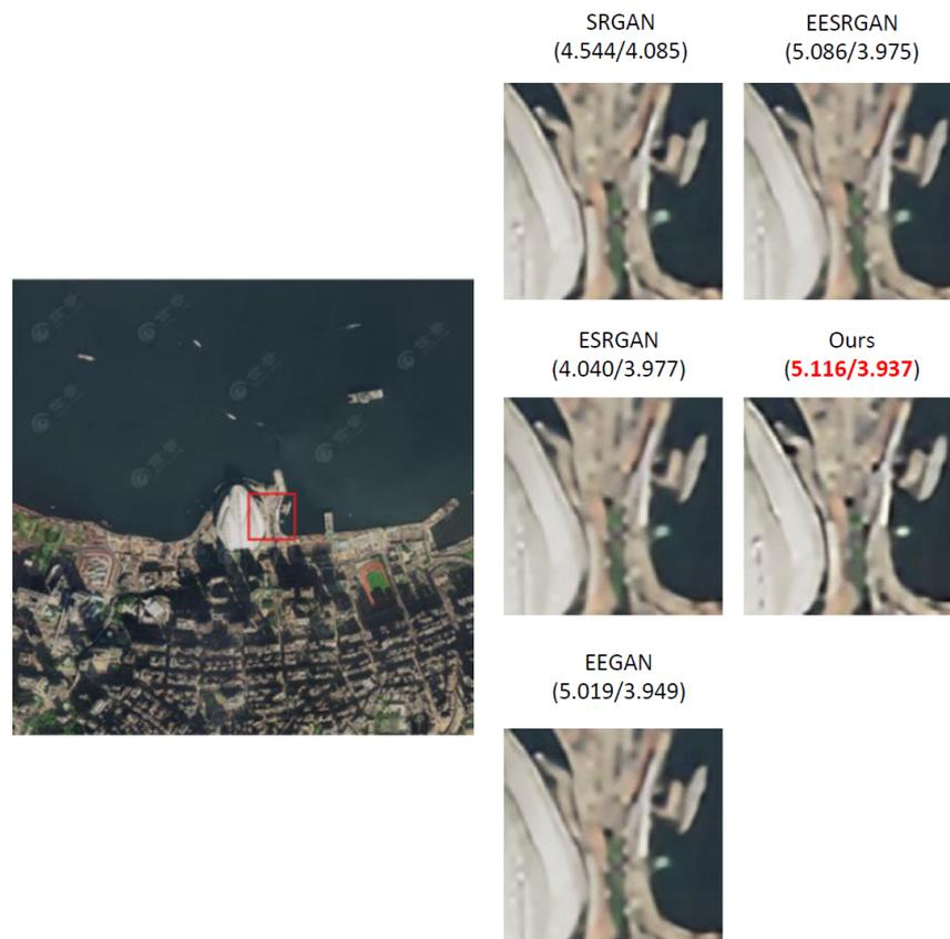
**Figure 15.** An enlarged partial view of the SR result of each method in the SpaceWill dataset—sample image 2, where the best results are shown in red font.
