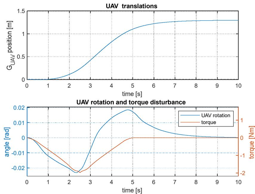
Figure 8. UAV horizontal translation (top) and rotation/torque disturbance (bottom) during the linear trajectory task for the 2-DOF trolley model with PID control assumption.
