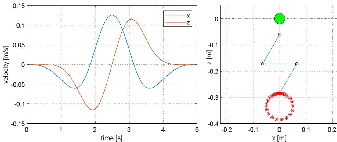
**Figure 4.** End-effector desired velocities for the circular trajectory (left) and initial configuration for a 3-DOF manipulator (right). The UAV base is the large green marker, joints are the black circles, links are the blue lines, and end-effector positions tracked are the red crosses.
