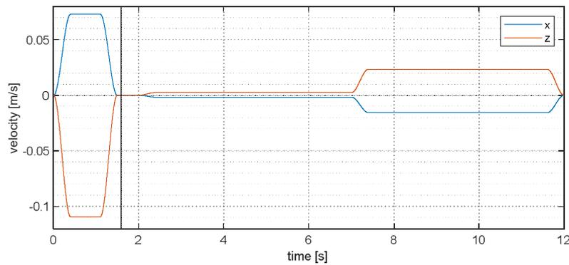
**Figure 21.** Desired end-effector velocities for the load picking task. The vertical gray line indicates the start time of contact.
