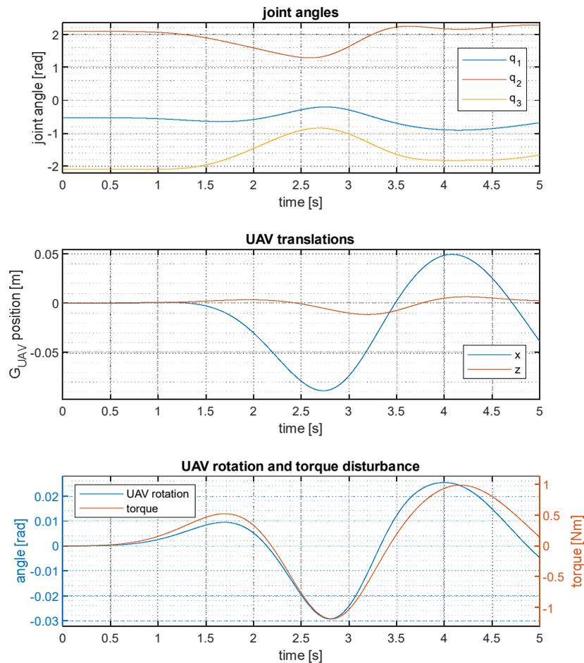
**Figure 15.** Manipulator (top) and UAV motions and torque disturbance (middle and bottom) for the 3-DOF UAM using the generalized Jacobian with external forces performing a circular trajectory task.
