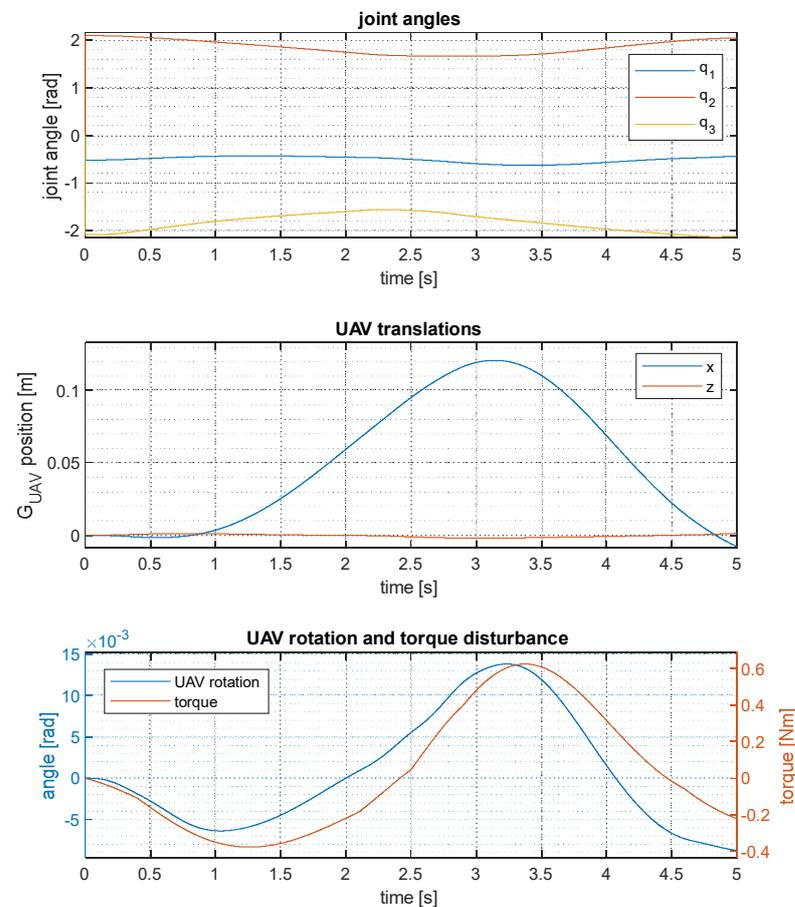
**Figure 13.** Manipulator (top) and UAV motions and torque disturbance (middle and bottom) for the 3-DOF UAM using the generalized Jacobian with external forces performing a linear trajectory task.
