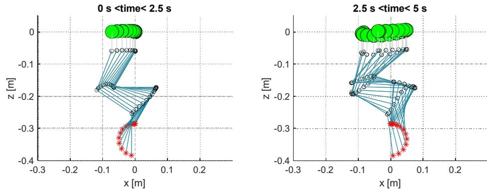
**Figure 14.** Stroboscopic trajectories for the first half (left) and second half (right) of the circular trajectory task for the 3-DOF redundant UAM using the generalized Jacobian with external forces. The UAV base is the large green marker, joints are the black circles, links are the blue lines, and end-effector positions tracked are the red crosses.
