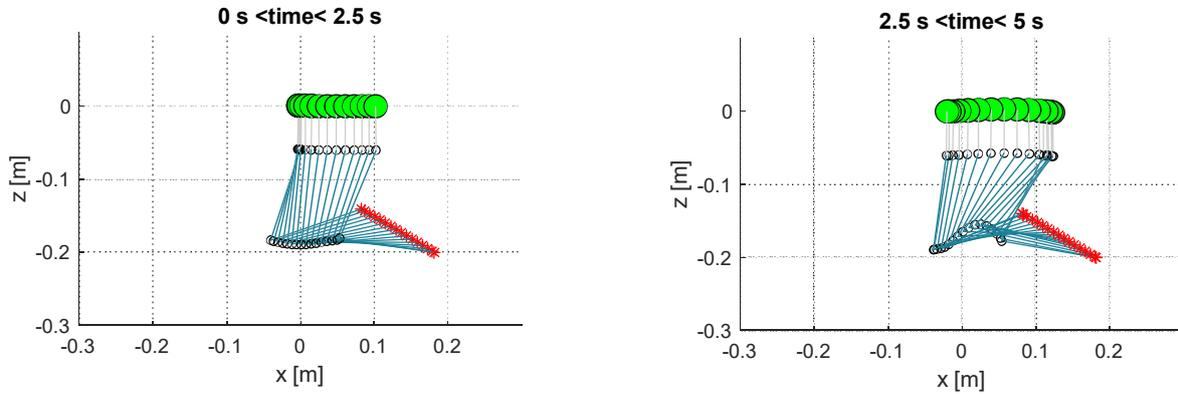
**Figure 10.** Stroboscopic trajectories for the first half (left) and second half (right) of the linear trajectory task for the 2-DOF UAM using the generalized Jacobian with external forces. The UAV base is the large green marker, joints are the black circles, links are the blue lines, and end-effector positions tracked are the red crosses.
