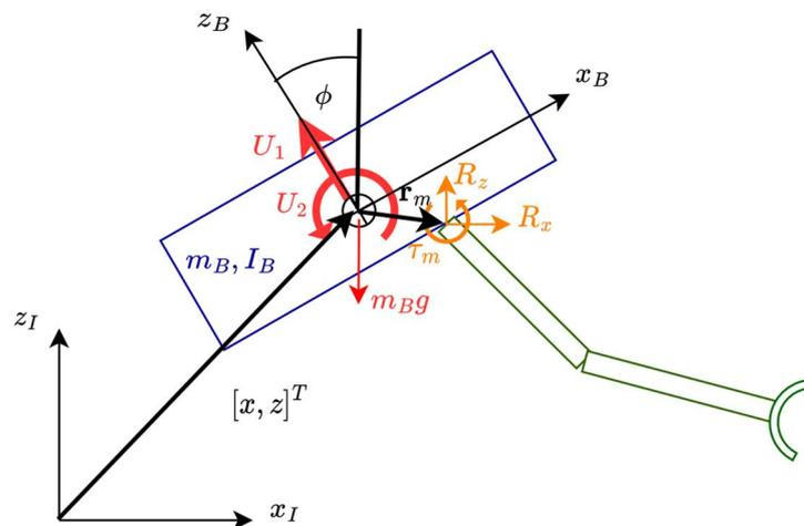
Figure 2. Coordinates and forces of the UAM. UAV forces/torques are in red and manipulator reaction forces/torques are in orange. The UAV is shown in blue and manipulator in green.
