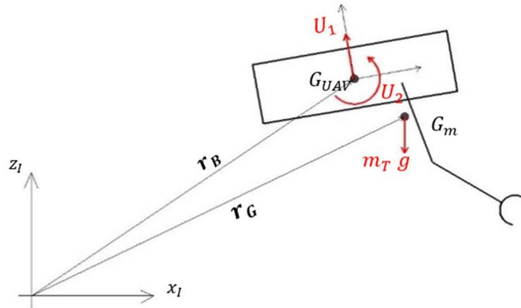
**Figure 9.** External forces on the UAM for the generalized Jacobian formulation.
