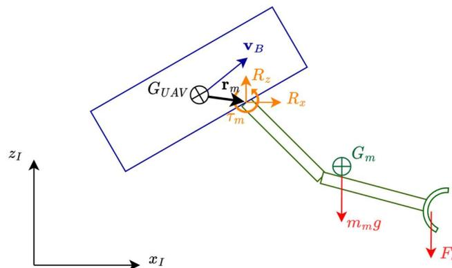
**Figure 16.** Forces and torques on the manipulator for the extended Jacobian formulation. Centers of gravity are the circles with crosses (black for the UAV, green for the manipulator), external forces are in red, reaction forces/torques in orange.
