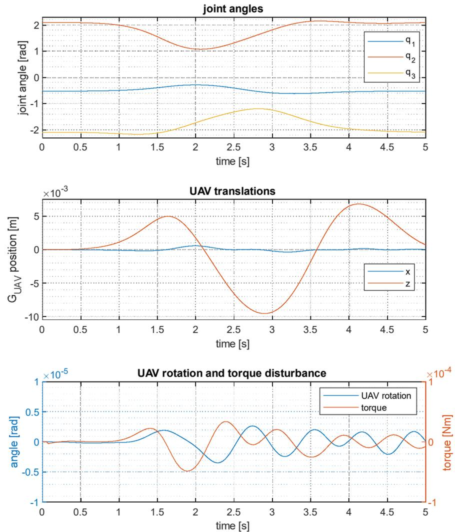
**Figure 20.** Manipulator (**top**) and UAV motions and torque disturbance (**middle** and **bottom**) for the circular trajectory task with the 3-DOF UAM using the extended generalized Jacobian.
