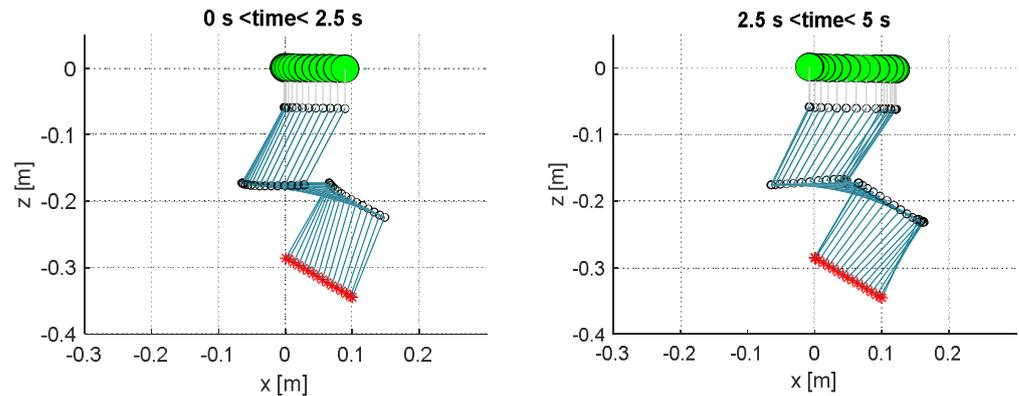
**Figure 12.** Stroboscopic trajectories for the first half (left) and second half (right) of the linear trajectory task for the 3-DOF redundant UAM using the generalized Jacobian with external forces. The UAV base is the large green marker, joints are the black circles, links are the blue lines, and end-effector positions tracked are the red crosses.
