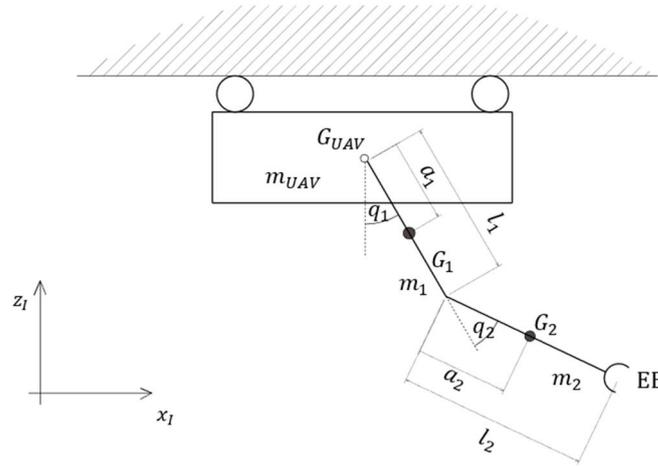
Figure 5. Model for the ideal 2-DOF trolley case.
