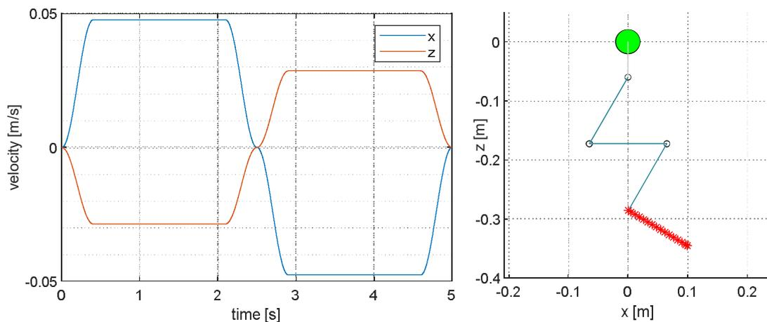
**Figure 3.** End-effector desired velocities for the line trajectory (left) and initial configuration for 3-DOF manipulator (right). The UAV base is the large green marker, joints are the black circles, links are the blue lines, and end-effector positions tracked are the red crosses.
