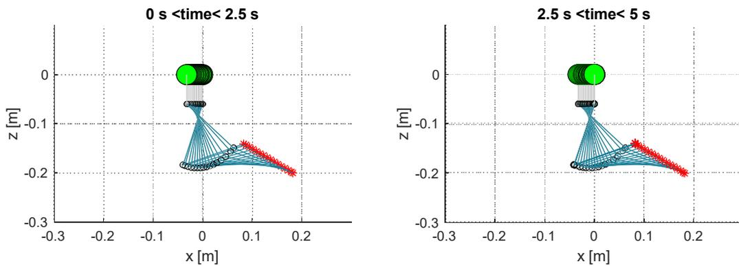
**Figure 6.** Stroboscopic trajectories for the first half (left) and second half (right) of the linear trajectory task for the 2-DOF trolley model and ideal control assumption. The UAV base is the large green marker, joints are the black circles, links are the blue lines, and end-effector positions tracked are the red crosses.
