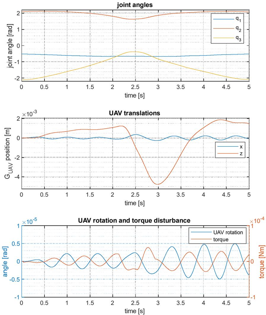
**Figure 18.** Manipulator (**top**) and UAV motions and torque disturbance (**middle** and **bottom**) for the linear trajectory task with the 3-DOF UAM using the extended Jacobian.
