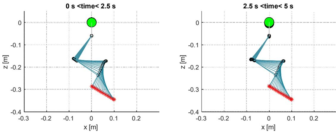
**Figure 17.** Stroboscopic trajectories for the first half (**left**) and second half (**right**) of the linear trajectory task for the 3-DOF redundant UAM using the extended Jacobian. The UAV base is the large green marker, joints are the black circles, links are the blue lines, and end-effector positions tracked are the red crosses.
