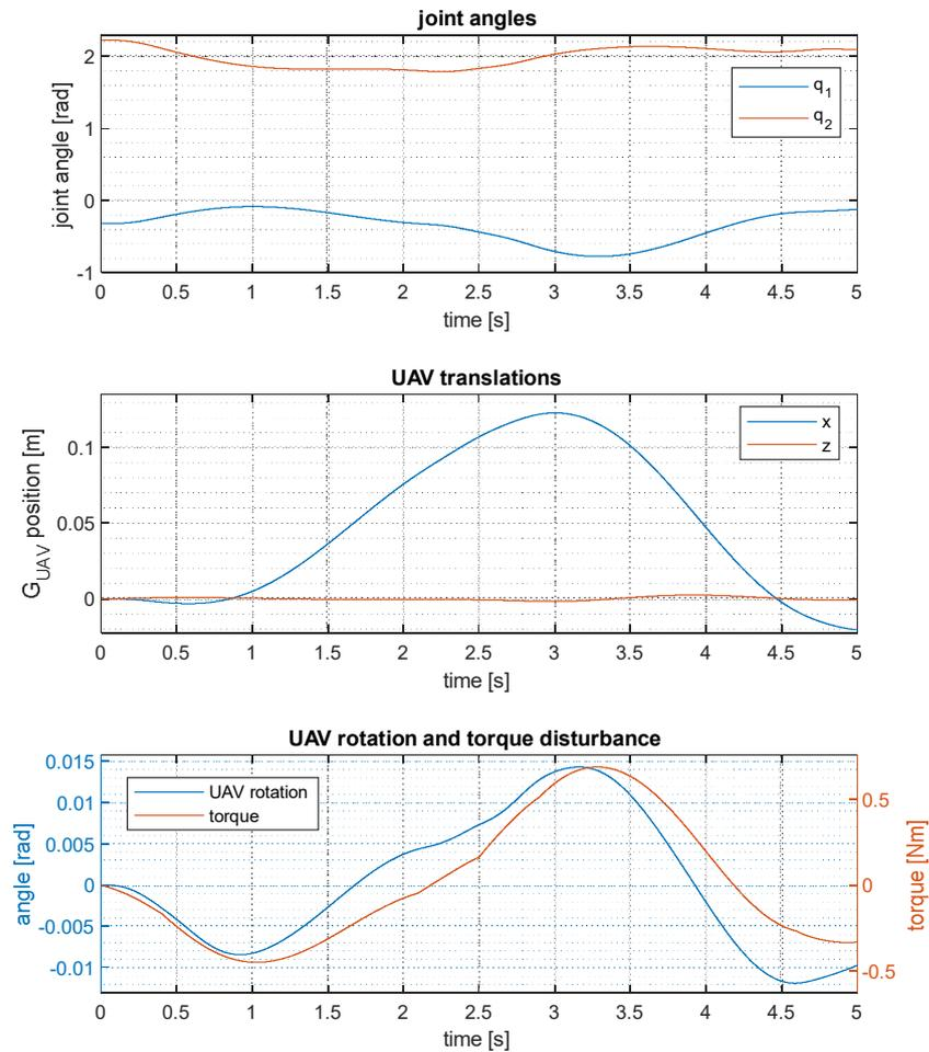
**Figure 11.** Manipulator (top) and UAV motions and torque disturbance (middle and bottom) for the 2-DOF UAM using the generalized Jacobian with external forces.
