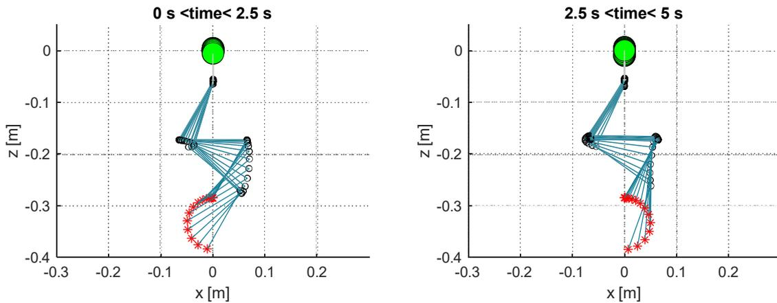
**Figure 19.** Stroboscopic trajectories for the first half (**left**) and second half (**right**) of the circular trajectory task for the 3-DOF redundant UAM using the extended generalized Jacobian. The UAV base is the large green marker, joints are the black circles, links are the blue lines, and end-effector positions tracked are the red crosses.
