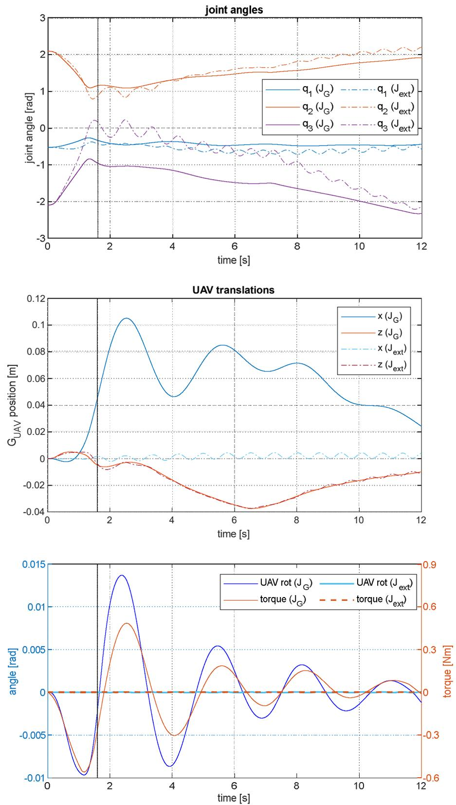
**Figure 23.** Comparison between generalized Jacobian with external forces ( $J_G$ ) and extended generalized Jacobian ( $J_{ext}$ ) solutions for the 3-DOF redundant UAM: manipulator motions (**top**), UAV translations (**middle**), UAV rotation and torque disturbance from the manipulator to the UAV (**bottom**). The vertical dark line indicates the start time of contact for the grasp.
