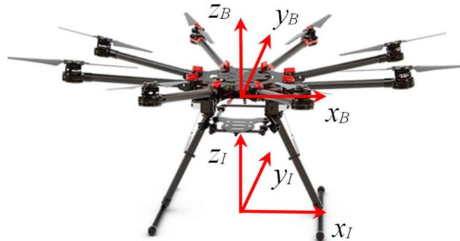
Figure 1. Illustration of reference frames for the UAV system (DJI S1000) [12].
