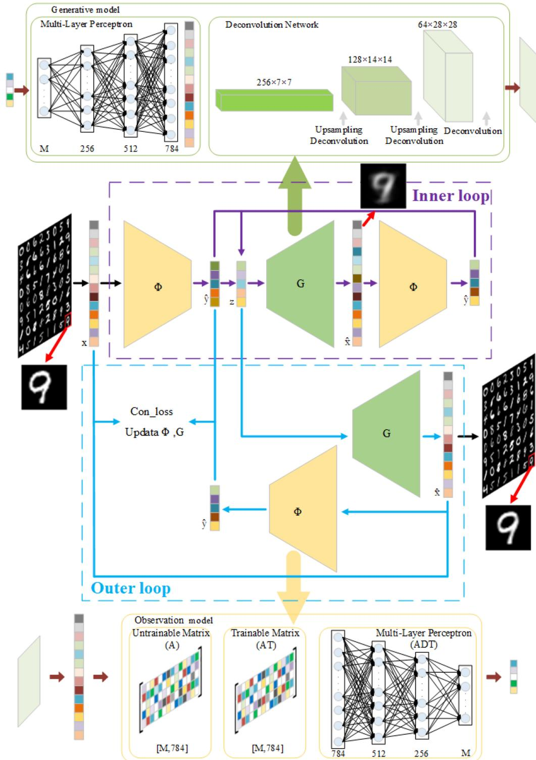
Figure 1. Block diagram to the E2E\_DCSGM structure.
