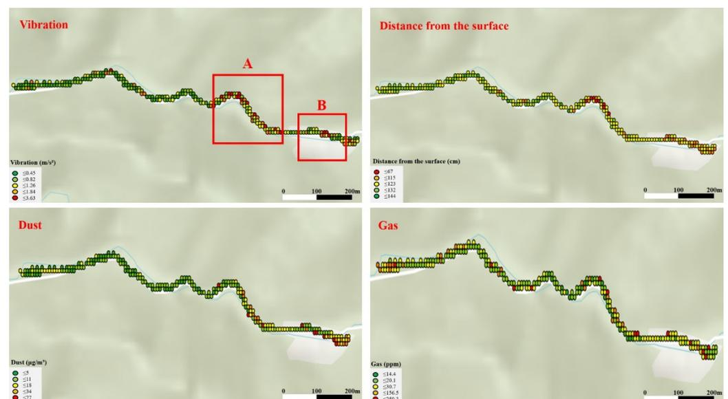
**Figure 11.** Analysis results of the spatial distributions of vibration, distance from the surface, dust concentration, and gas concentration. Sections A and B have rough road conditions.
