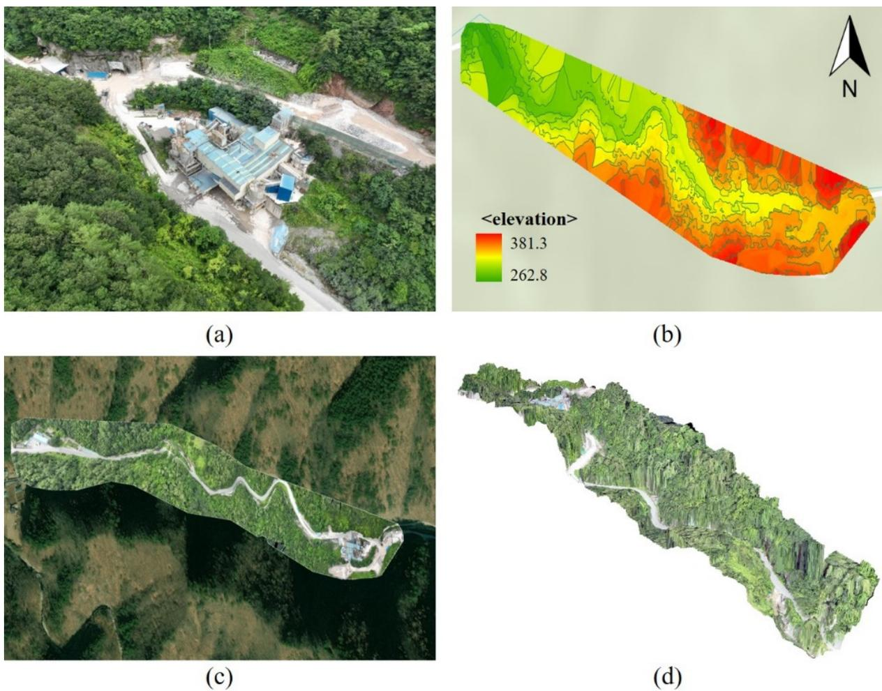
**Figure 1.** (a) Panoramic image, (b) DSM, (c) orthoimage, and (d) three-dimensional image of Taeyoung EMC's Samdo mine.
