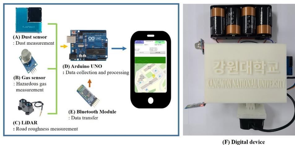
Figure 3. (A) Dust sensor, (B) gas sensor, (C) LiDAR, (D) Arduino Uno, (E) Bluetooth module, and (F) a digital device that combines Arduino and sensors.
