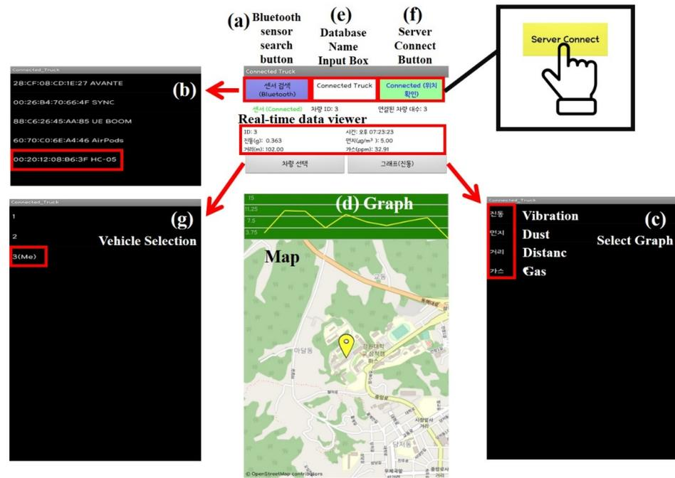
Figure 4. Interface of developed smartphone application. (a) Bluetooth sensor search button, (b) searched Bluetooth modules, (c) graph selection window, (d) selected graph, (e) database name input box, (f) server connect button, and (g) vehicle selection window.
