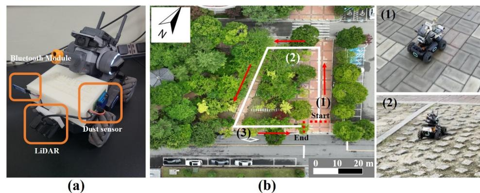
**Figure 6.** Images of (a) RoboMaster S1 and (b) preliminary test site (Samcheok Campus, Kangwon National University).
