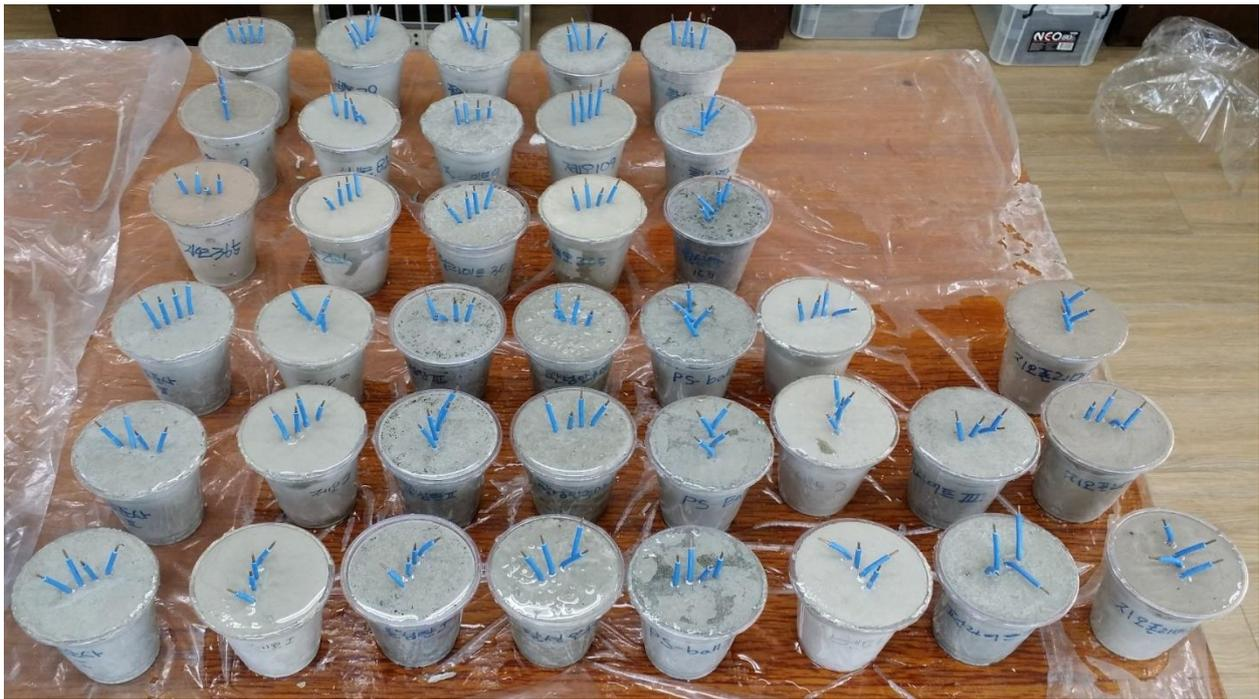
**Figure 1.** Prepared cup-shaped mortar specimens for resistivity measurement.
