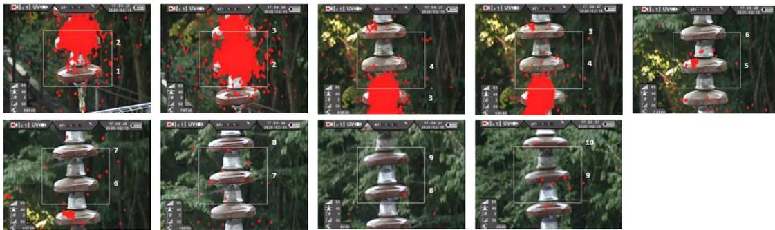
**Figure 2.** UV connection between the cup-and-pin insulators that had reached 40% of string length. The first cup-and-pin insulator was closest to the energized terminal.
