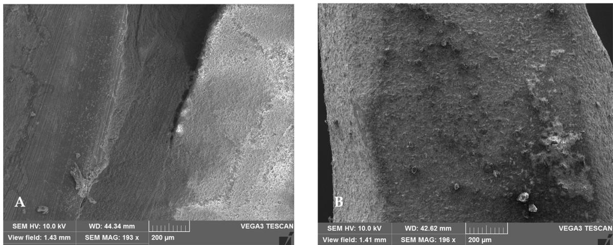
**Figure 10.** Scanning-electron-microscope image of (A) Sectioned root canal, and (B) displaced post, at 200× magnification, showing cohesive failure mode in Group 2 (CMTPCs) sample at root/post interface.
