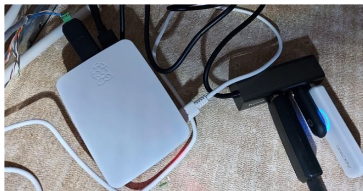
Figure 13. Edge: Raspberry Pi with dongle sticks.
