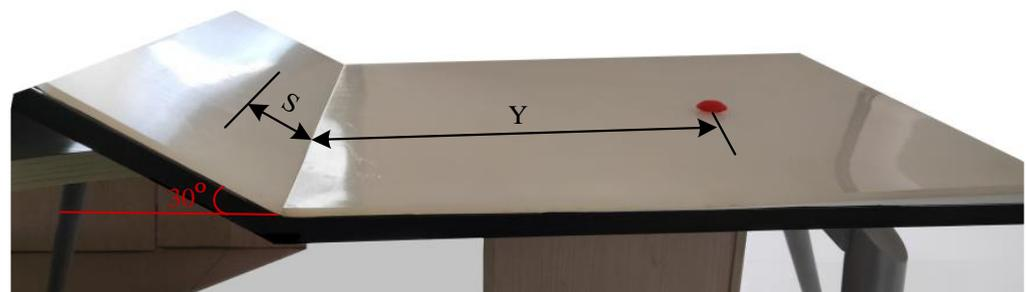
**Figure 8.** Physical experiment for calibrating the rolling friction coefficient of fresh goji berry–silicone rubber material.
