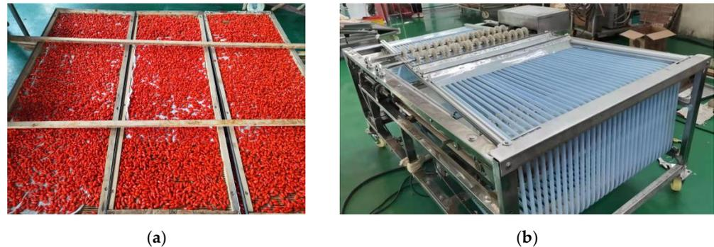
**Figure 17.** Experimental equipment for field tests. (a) The experiment target is mature fresh goji berries of Ningqi No.5; (b) A variable gap-type fresh goji berry grading machine.
