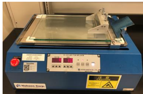
Figure 1. Prepare silicone conformal coating A and B films with an auto film applicator.
