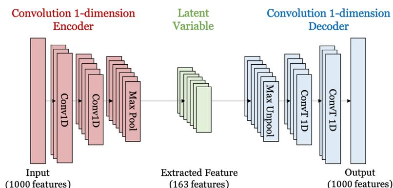
**Figure 3.** Structure of autoencoder for feature extraction.
