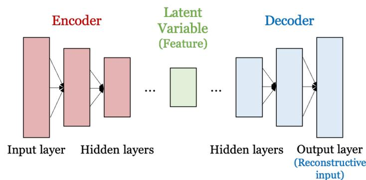
**Figure 1.** Structure of the autoencoder.
