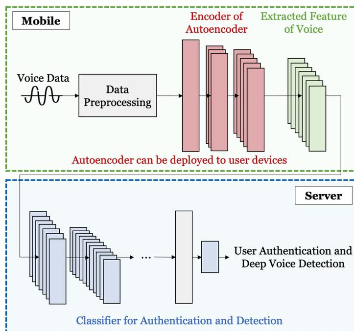
Figure 2. Diagram of proposed method.
