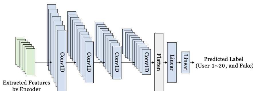
Figure 4. Structure of classifier for authentication and detection.
