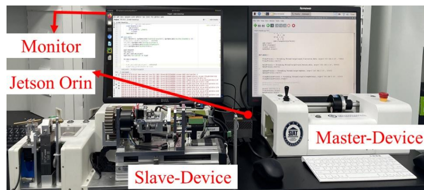
Figure 15. The hardware setup for experimental validation of the neural-based models within the RCS using Jetson Orin as the slave device's processor.
