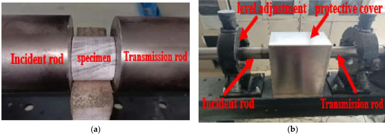
**Figure 5.** Schematic diagram of specimen loading. (a) Schematic diagram of loading; (b) Schematic diagram of loading device.
