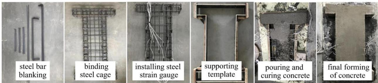
**Figure 2.** The specimen preparation process.
