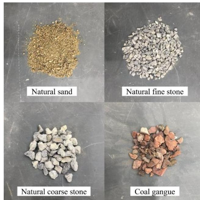
**Figure 3.** Concrete aggregate.
