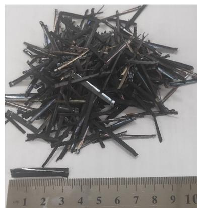
**Figure 1.** Mill steel fiber.
