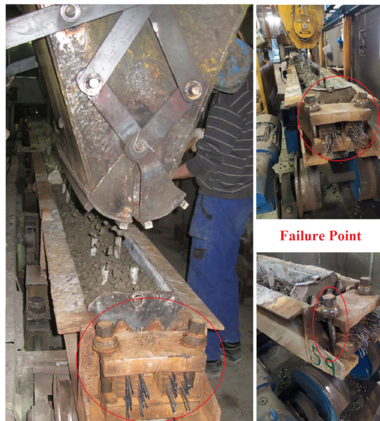
Figure 1. The sleeper mold and the failure point.
