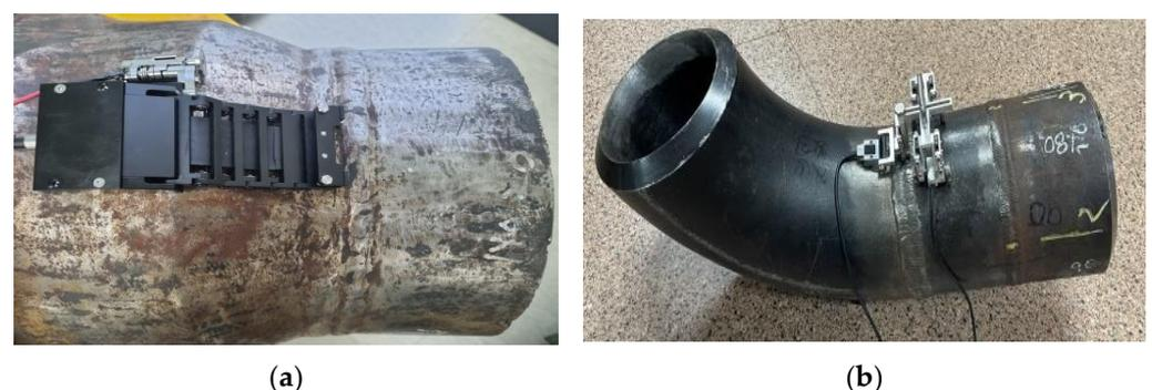
**Figure 16.** Semi-automatic scanner employed an actual specimen: (a) scanner with FPAPr and encoder attached; (b) scanner with PA probe and encoder attached.
