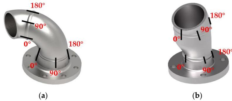
**Figure 20.** Angles for each inspection position on the experimental welding test pieces: (a) 100 mm curvature pipe with elbow–flange construction geometry; (b) 75 mm, 100 mm curvature pipe with elbow–flange–reducer construction geometry.
