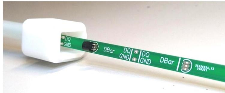
Figure 5. Sensors installed on a PCB module.
