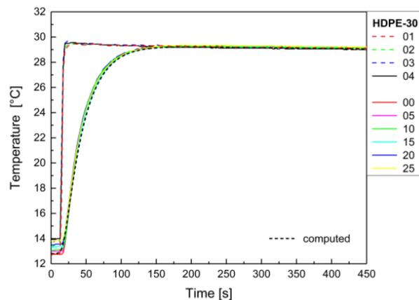
**Figure 17.** Time-history of measured temperatures and the temperatures computed in the probe axis (measurement A—water bath temperature of 30 °C/probe 2).
