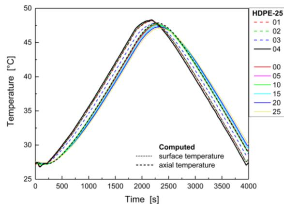
**Figure 24.** Time-history of measured temperatures and computed surface and axial temperatures (measurement B—temperature increase in climate chamber by 25 °C/probe 2).
