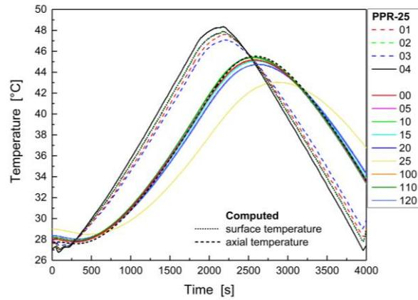
**Figure 21.** Time-history of measured temperatures and computed surface and axial temperatures (measurement B—temperature increase in climate chamber by 25 °C/probe 1).
