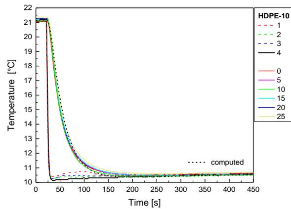
**Figure 18.** Time-history of measured temperatures and the temperatures computed in the probe axis (measurement A—water bath temperature of 10 °C/probe 2).
