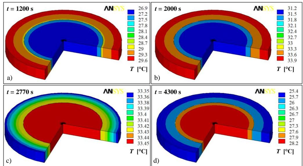
Figure 11. Temperature distribution in probe 1 at chosen times during its heating by 10  $^{\circ}\text{C}$  and subsequent cooling in the climate chamber, (a)  $t = 1200$  s, (b)  $t = 2000$  s, (c)  $t = 2770$  s and (d)  $t = 4300$  s.
