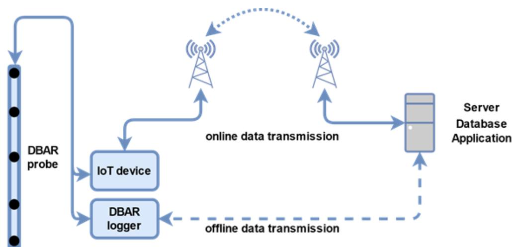
Figure 6. System architecture block diagram.
