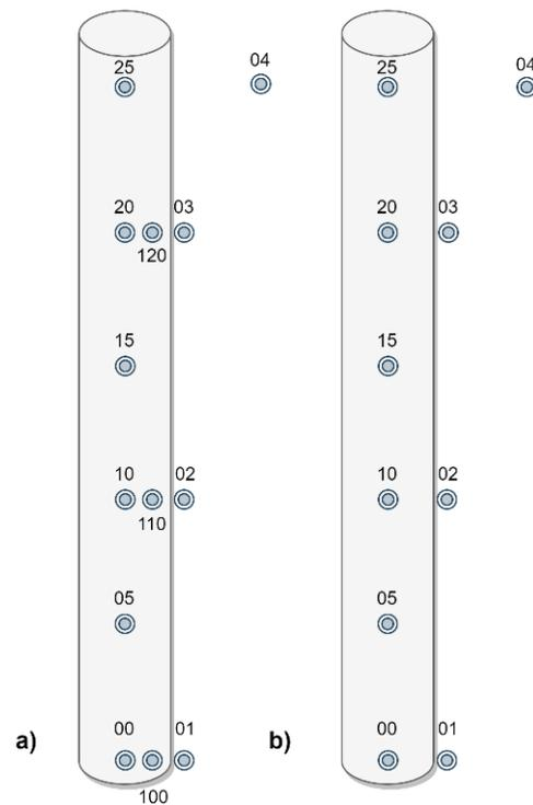
**Figure 7.** Experimental probes: (a) PPR and (b) HDPE.
