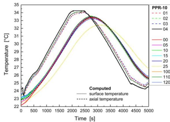
**Figure 19.** Time-history of measured temperatures and computed surface and axial temperatures (measurement B—temperature increase in climate chamber by 10 °C/probe 1).
