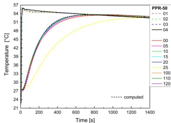
**Figure 13.** Time-history of measured temperatures and the temperatures computed in the probe axis (measurement A—water bath temperature of 55 °C/probe 1).
