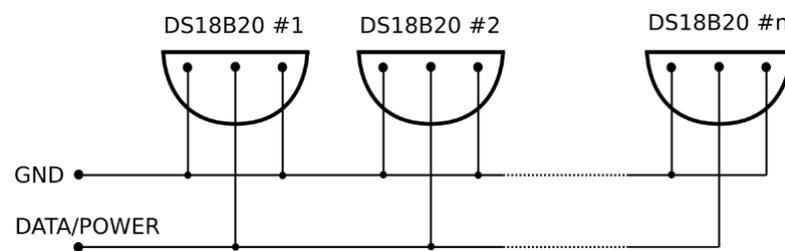
**Figure 1.** Parasitic connection of sensors.
