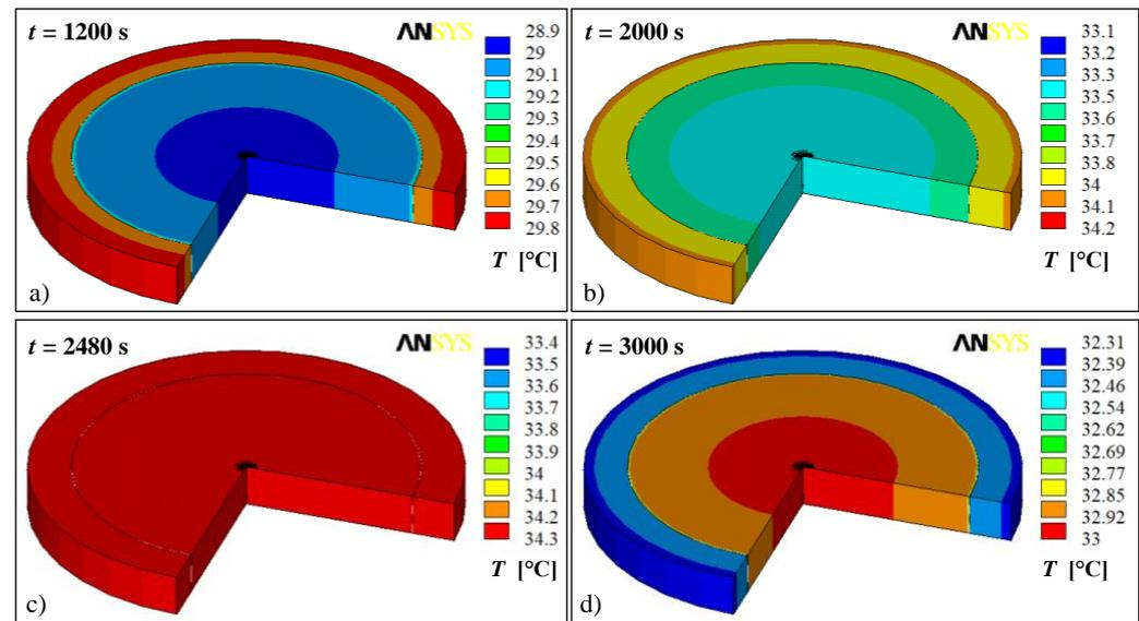
Figure 12. Temperature distribution in probe 2 at chosen times during its heating by 10  $^{\circ}\text{C}$  and subsequent cooling in the climate chamber, (a)  $t = 1200$  s, (b)  $t = 2000$  s, (c)  $t = 2480$  s and (d)  $t = 3000$  s.
