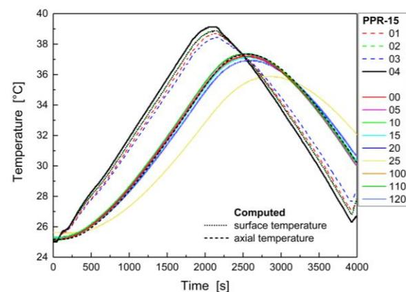
**Figure 20.** Time-history of measured temperatures and computed surface and axial temperatures (measurement B—temperature increase in climate chamber by 15 °C/probe 1).
