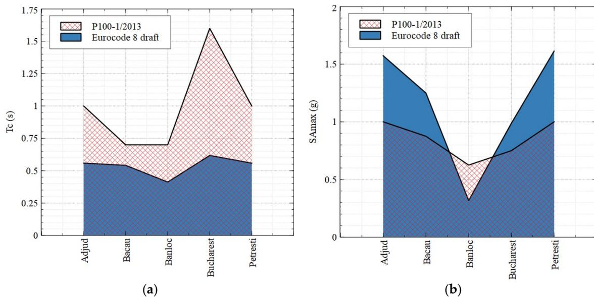
**Figure 6.** (a) A comparison between the control period  $T_C$  from P100-1/2013 [29] and based on Eurocode 8 draft revision [1] for category F sites; (b) a comparison between the maximum spectral acceleration from P100-1/2013 [29] and based on Eurocode 8 draft revision [1] for category F sites.
