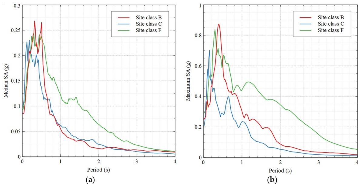
**Figure 2.** (a) The median spectral accelerations as a function of the site class; (b) the maximum spectral accelerations as a function of the site class.
