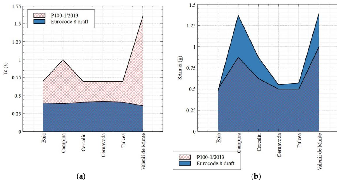
**Figure 4.** (a) A comparison between the control period  $T_C$  from P100-1/2013 [29] and based on Eurocode 8 draft revision [1] for category B sites; (b) a comparison between the maximum spectral acceleration from P100-1/2013 [29] and based on Eurocode 8 draft revision [1] for category B sites.
