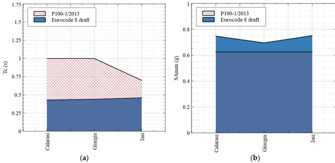
**Figure 5.** (a) A comparison between the control period  $T_C$  from P100-1/2013 [29] and based on Eurocode 8 draft revision [1] for category C sites; (b) a comparison between the maximum spectral acceleration from P100-1/2013 [29] and based on Eurocode 8 draft revision [1] for category C sites.
