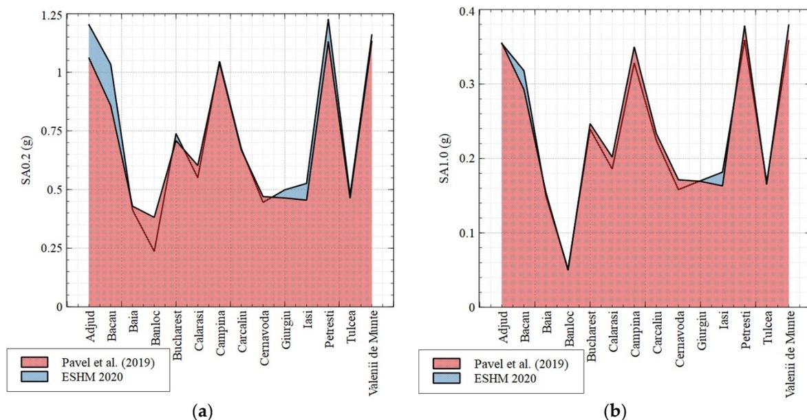
**Figure 3.** (a) A comparison between the spectral accelerations that had a mean return period of 475 years for rock conditions for  $T = 0.2$  s obtained from the seismic hazard model of Pavel et al. [27] and from the ESHM 2020 model [26]; (b) a comparison between the spectral accelerations for rock conditions for  $T = 1.0$  s obtained from the seismic hazard model of Pavel et al. [27] and from the ESHM 2020 model [26].
