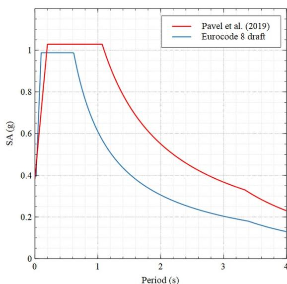
**Figure 10.** A comparison between the design acceleration response spectra for Bucharest computed using the site amplification proposed by Pavel et al. [4] and the site amplifications from the Eurocode 8 draft revision [1].
