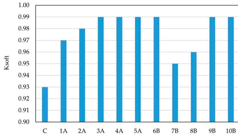
**Figure 11.** Softening coefficients of experimental compositions of geopolymer fine-grained concrete.
