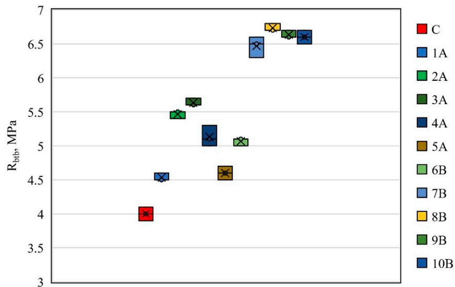
Figure 8. Bending tensile strength of fine-grained geopolymer concrete.
