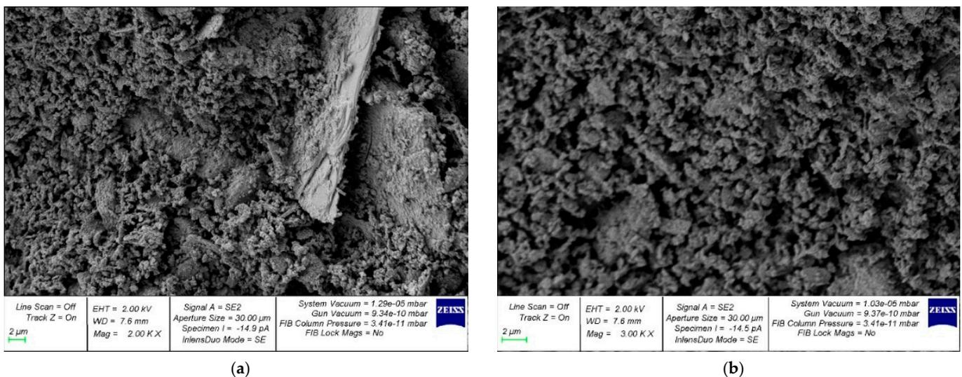
**Figure 12.** Microstructure of the geopolymer composite at the age of 28 days: (a) composition of type C; (b) composition of type 8B.
