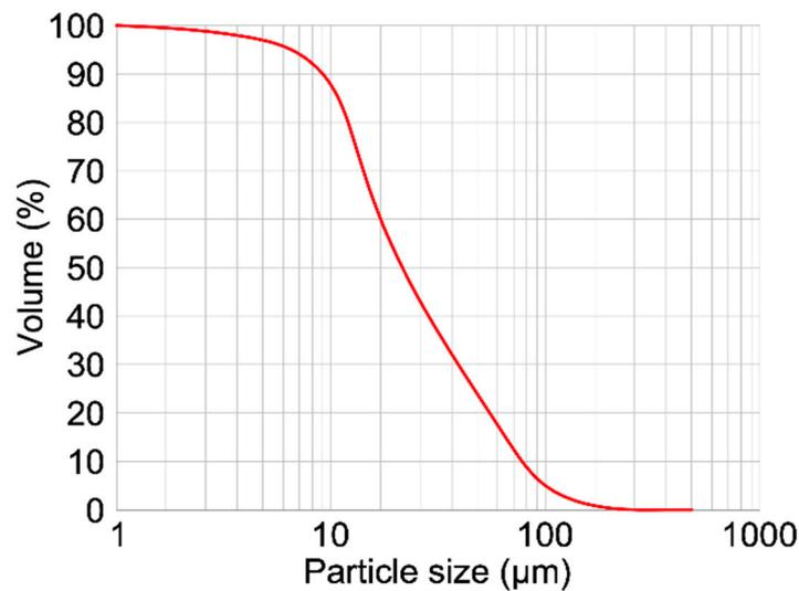
Figure 2. The size distribution curve of potassium feldspar grade FK-100.
