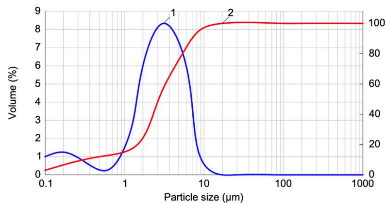
Figure 3. Curve of distribution of Km-2 grade micro calcite particles by size: 1—curve of the partial distribution of particles of a certain size (particle size) in percentage (along the left ordinate); 2—curve of the total distribution of particles as a percentage (on the right axis of ordinates).
