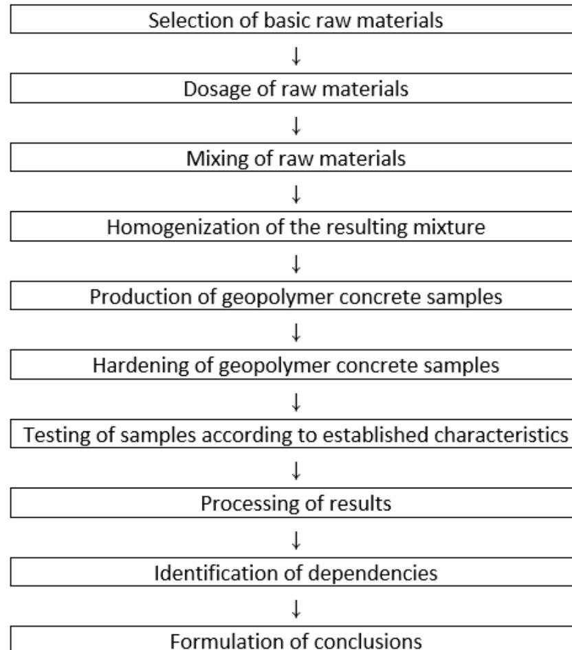
**Figure 4.** Step-by-step algorithm of the research methodology.
