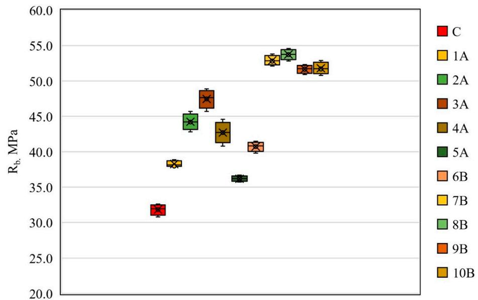
Figure 9. Strength of sample cubes after heat treatment (drying).
