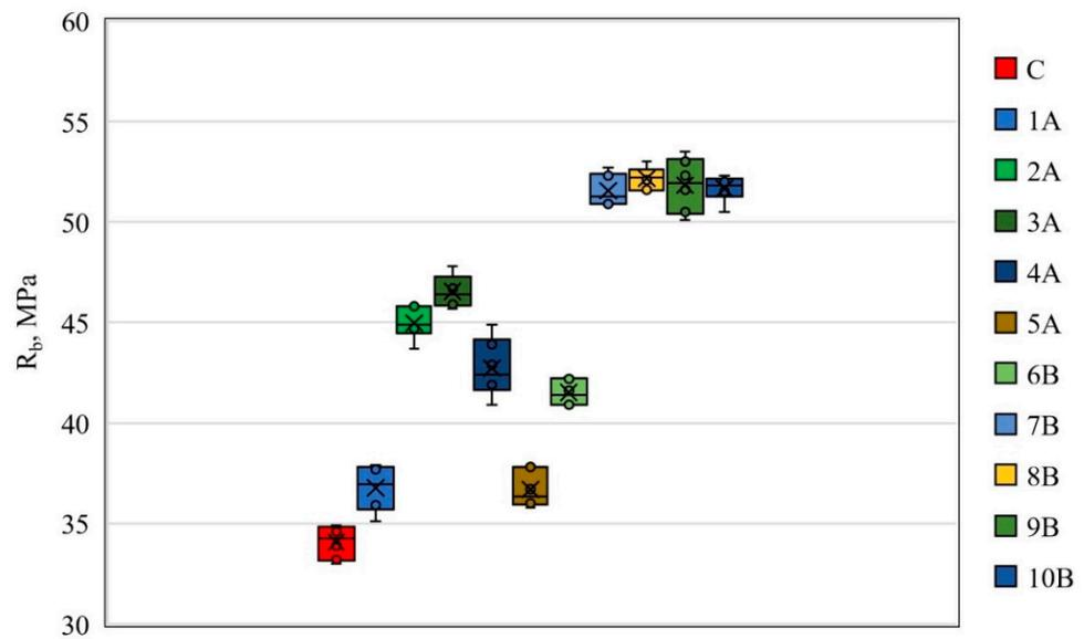
Figure 7. Compressive strength of fine-grained geopolymer concrete.
