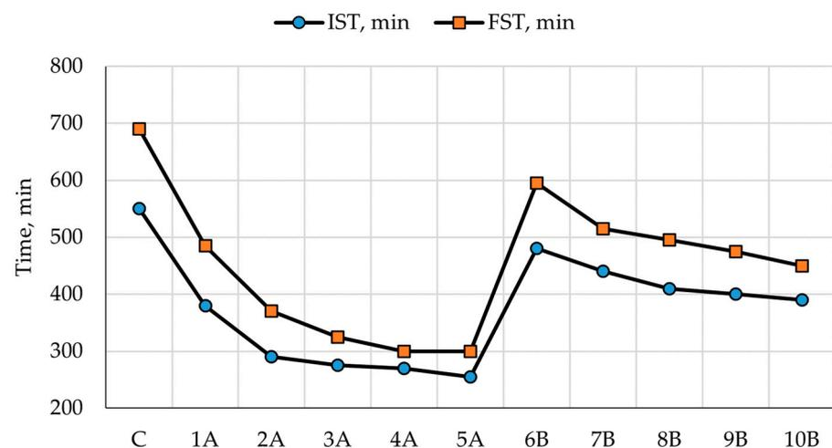
**Figure 6.** Dependence of changes in IST and FST on the content of stone flour: IST—initial setting time, FST—final setting time, C—control composition (without stone flour content), 1A–5A—marking of formulations with the addition of stone flour in the form of micro calcite, 6B–10B—marking of formulations with the addition of stone flour in the form of potassium feldspar.
