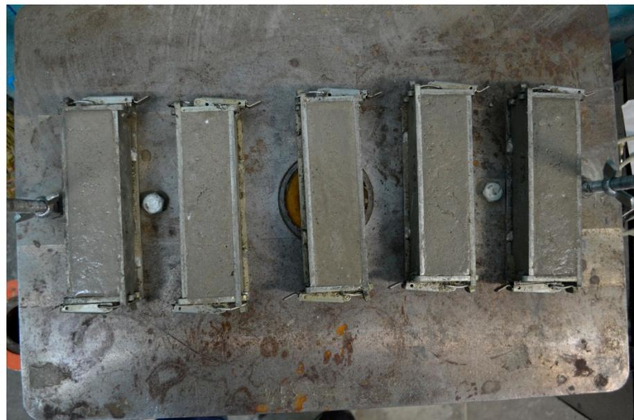
**Figure 5.** The process of vibration compaction of samples of geopolymer fine-grained concrete.
