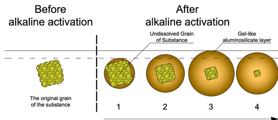
**Figure 13.** Phenomenological model of the formation of the system “gel layer–undissolved grain of material” in the process of alkaline activation.
