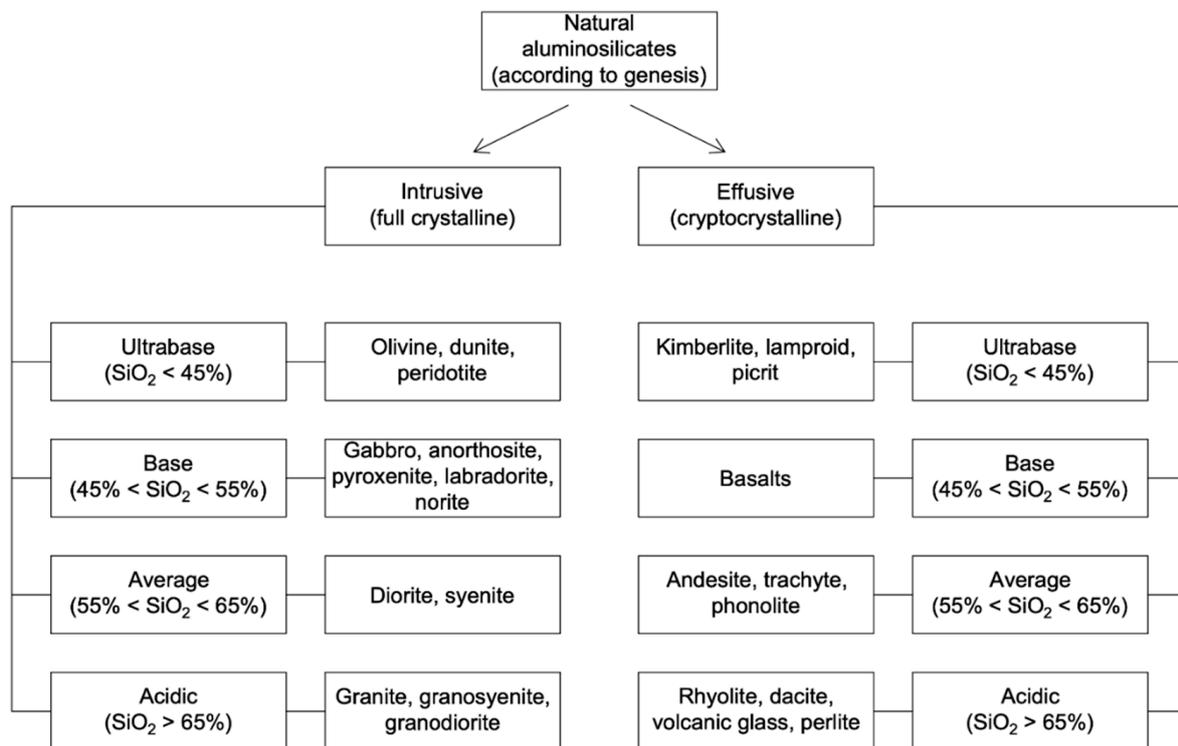
**Figure 1.** Classification of natural aluminosilicates.
