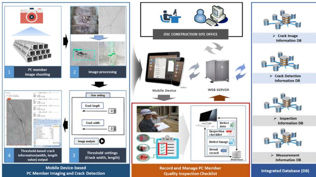
Figure 12. Conceptual diagram of the automated PC member crack detection system.
