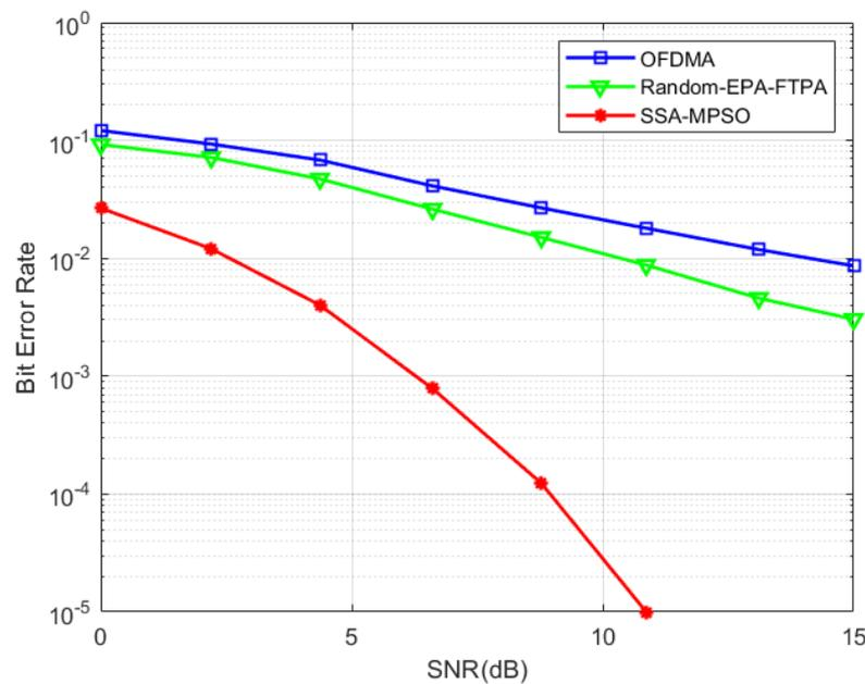
Figure 8. Bit error rate versus SNR.
