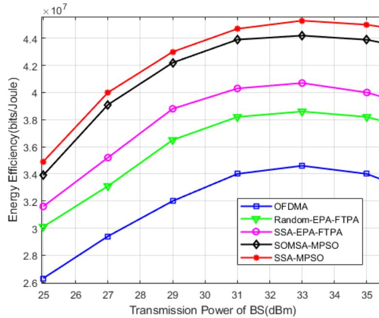
Figure 5. Energy efficiency versus maximum transmission power of BS.
