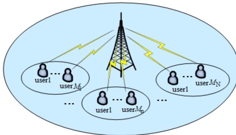
Figure 1. Downlink multicarrier NOMA system model.
