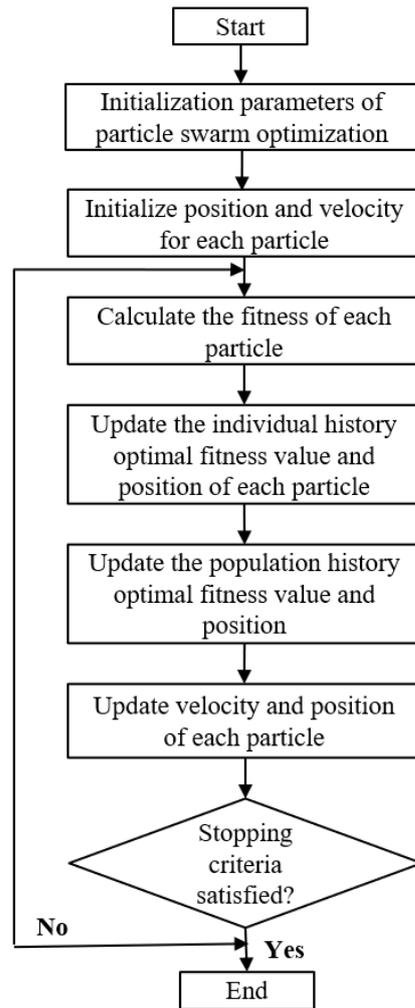
Figure 2. Flow chart of particle swarm optimization.
