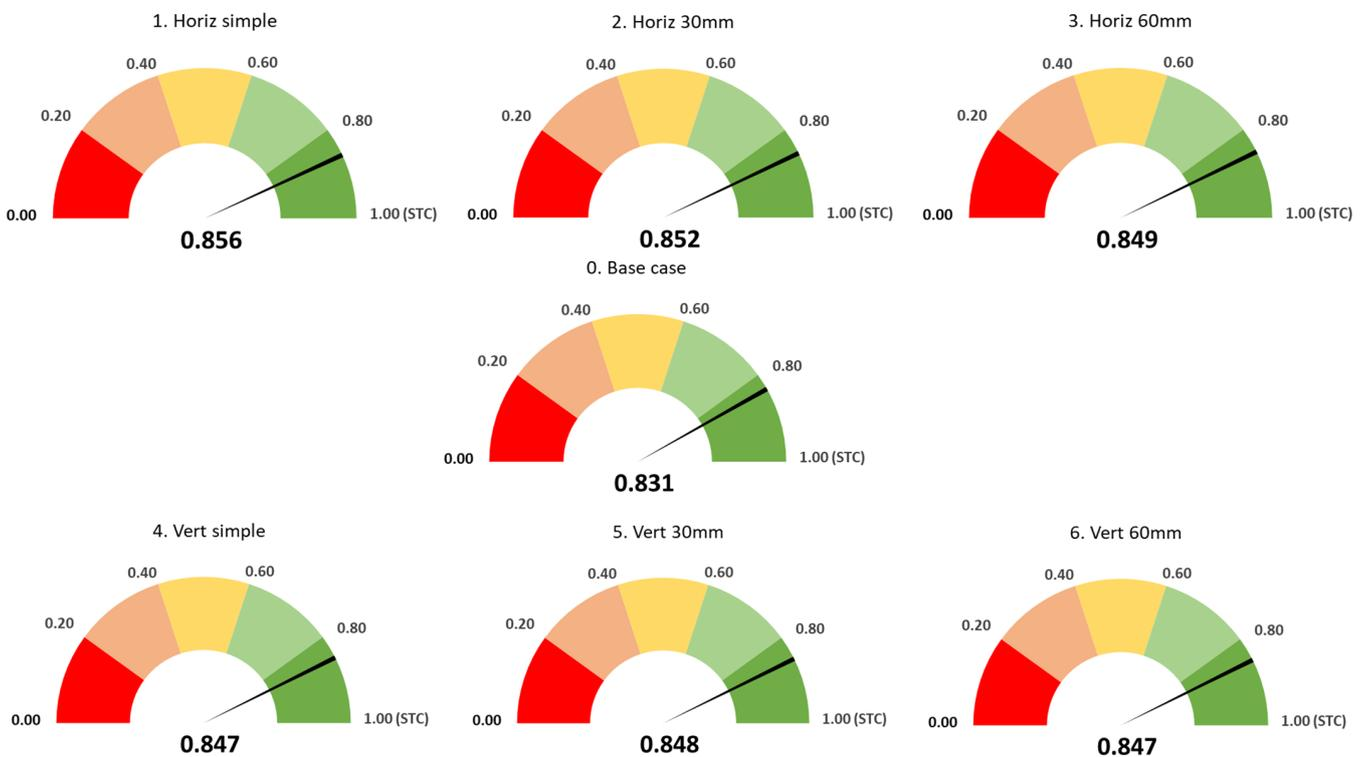
Figure 12. Normalized power production for front wind,  $v_{front} = 1 \text{ m/s}$ ,  $t_{air} = 35$ ,  $G = 1000 \text{ W/m}^2$ .
