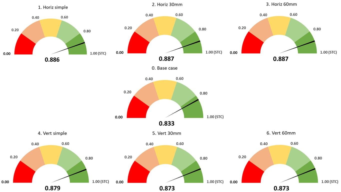
Figure 11. Normalized power production for back wind,  $v_{back} = 1 \text{ m/s}$ ,  $t_{air} = 35$ ,  $G = 1000 \text{ W/m}^2$ .
