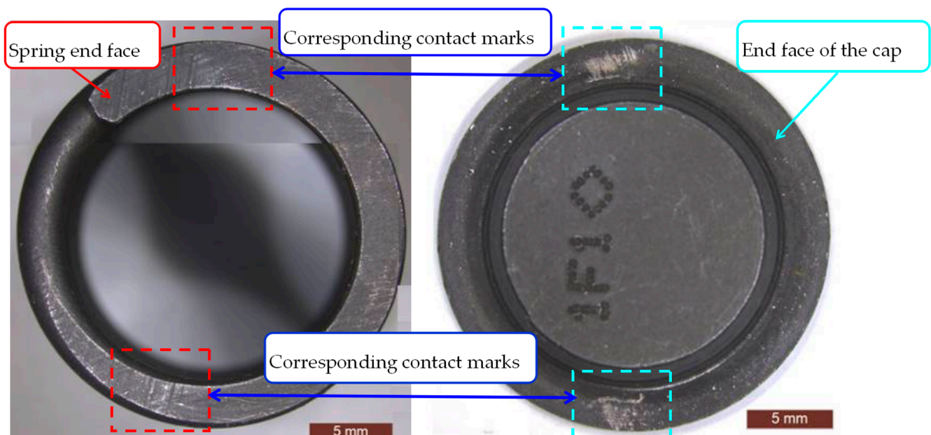
Figure 15. Two contact marks in the end face of the spring and the cap.
