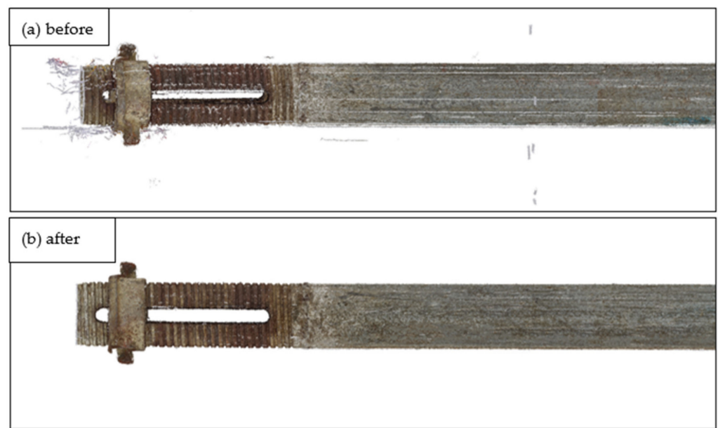
Figure 18. Noise removal. (a) Before, (b) after.
