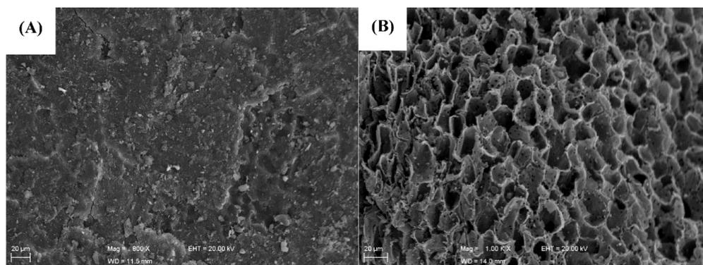
**Figure 2.** SEM micrographs ( $\times 800$  and  $\times 1000$ ) of (A) an in natura pecan shell (PS); and (B) the biosorbent (PSB).
