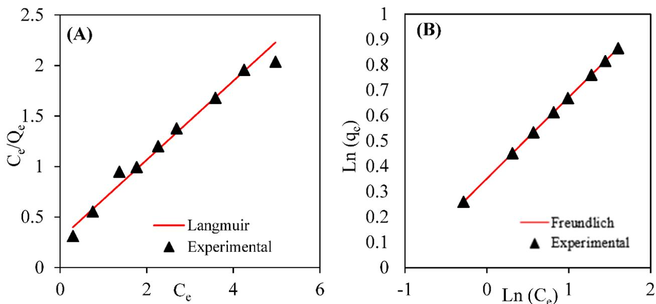
**Figure 6.** Linear plots of (A) Langmuir and (B) Freundlich isotherm models for the CPX biosorption by PSB.
