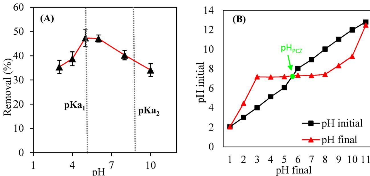
Figure 5. (A) Effect of pH on the removal capacity of the CPX and (B) the zero charge point pH.
