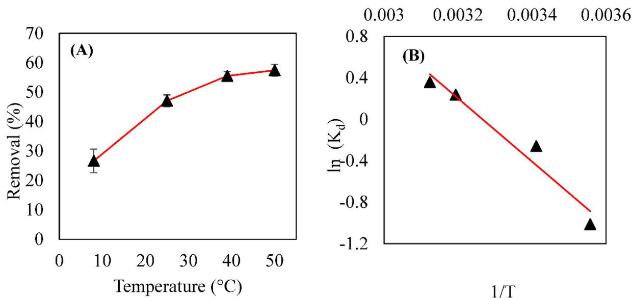
**Figure 7.** (A) Effects of temperature on CPX removal and (B) the van't Hoff graph for the system.
