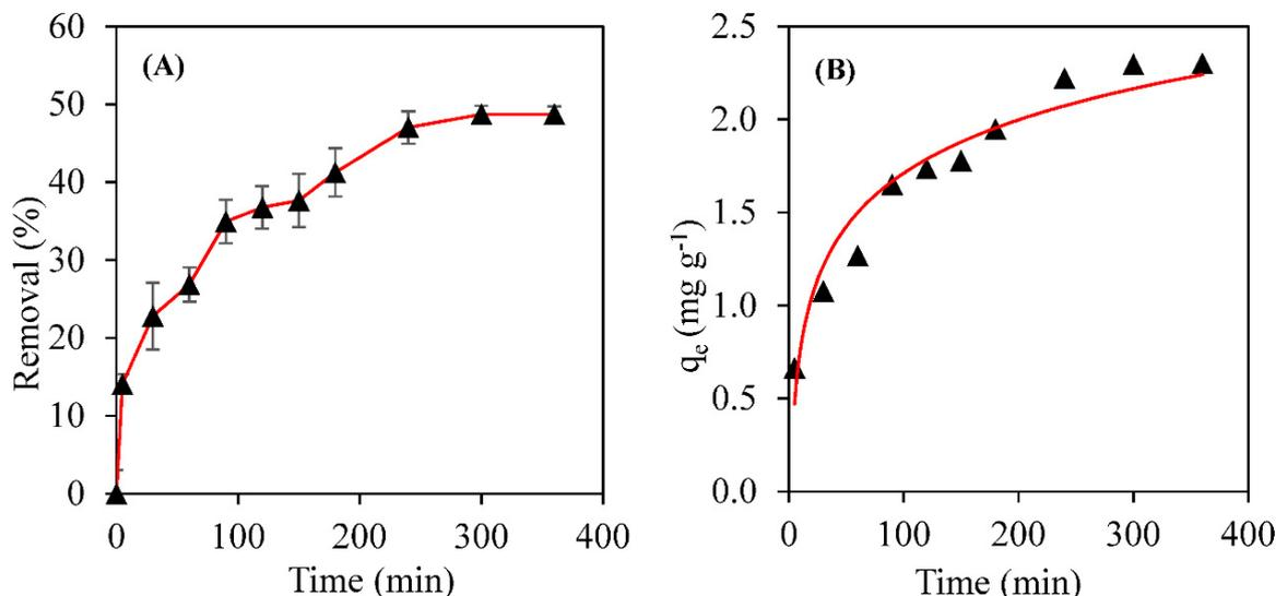
**Figure 3.** Equilibrium time for the CPX antibiotic. (A) the percentage of removal as a function of time; and (B) the amount adsorbed as a function of time.
