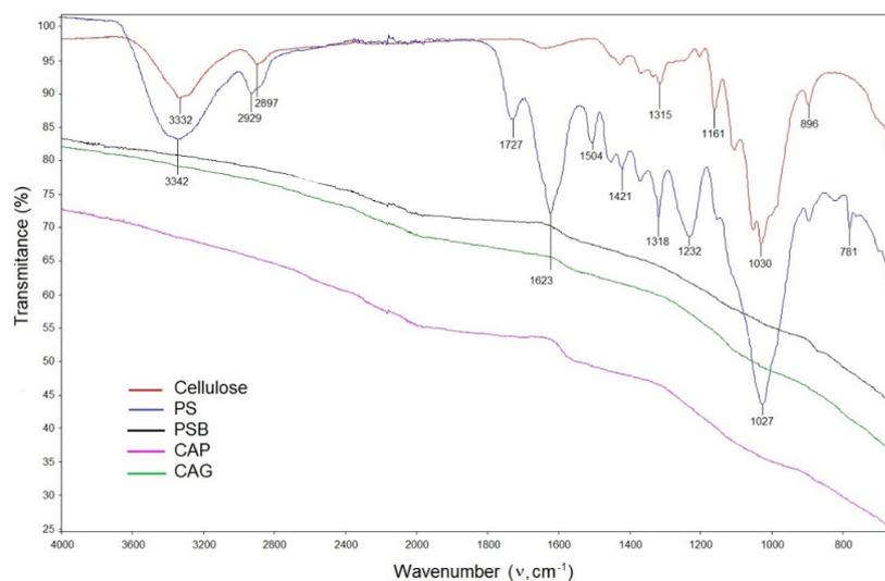
**Figure 1.** Characterization of the biochar via FT-IR for the PS, PSB, CAP, CAG and cellulose.
