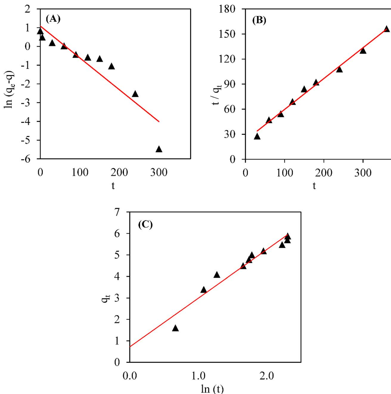
**Figure 4.** Linear plots of the (A) pseudo-first order kinetic model, (B) pseudo-second order kinetic model, and (C) Elovich model for ciprofloxacin adsorption by the biosorbent made of pecan shells.
