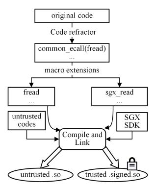
Figure 2. The backward-compatible compilation model for refactoring the code of a DNS resolver.
