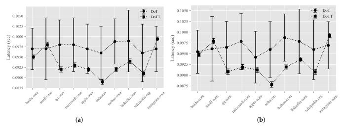
**Figure 6.** Performance evaluation of caching the resolved results between DoT and DoTT. (**a**) Caching 10 results, (**b**) caching 100 results.
