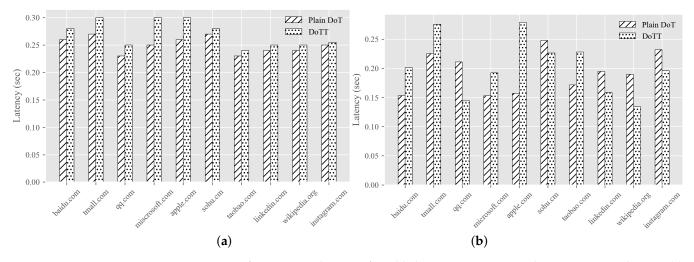
**Figure 5.** Performance evaluation of establishing TLS connections between DoT and DoTT. (**a**) Establishing TLS connections for each new request, and (**b**) reusing the existing connections for new requests.
