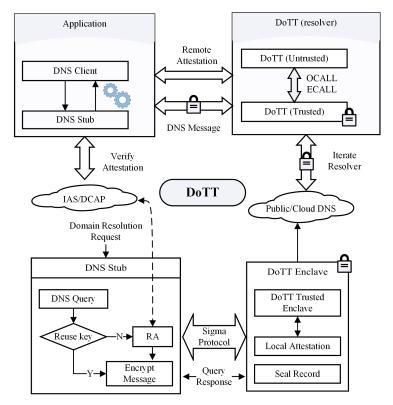
Figure 1. DoTT: The privacy enhancement framework for DNS based on TEE (Intel SGX).
