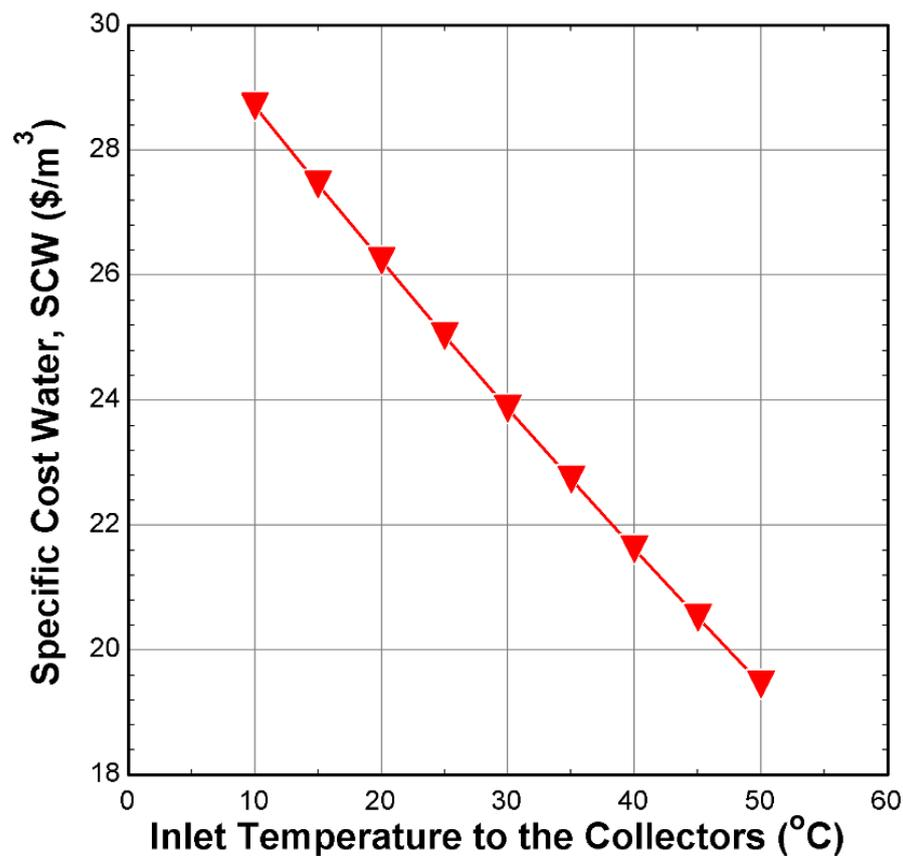
**Figure 8.** Effect of inlet water temperature to the collectors on SCW. The triangles represent the specific cost water values under the variation of collectors' temperature.
