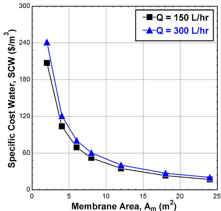
Figure 7. Effect of membrane area on Specific Cost Water (SCW) for different flow rates.
