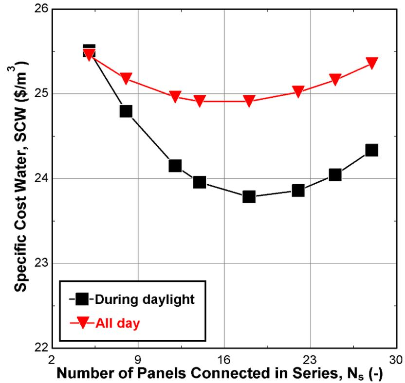
Figure 11. The SCW at different number of panels connected in series.
