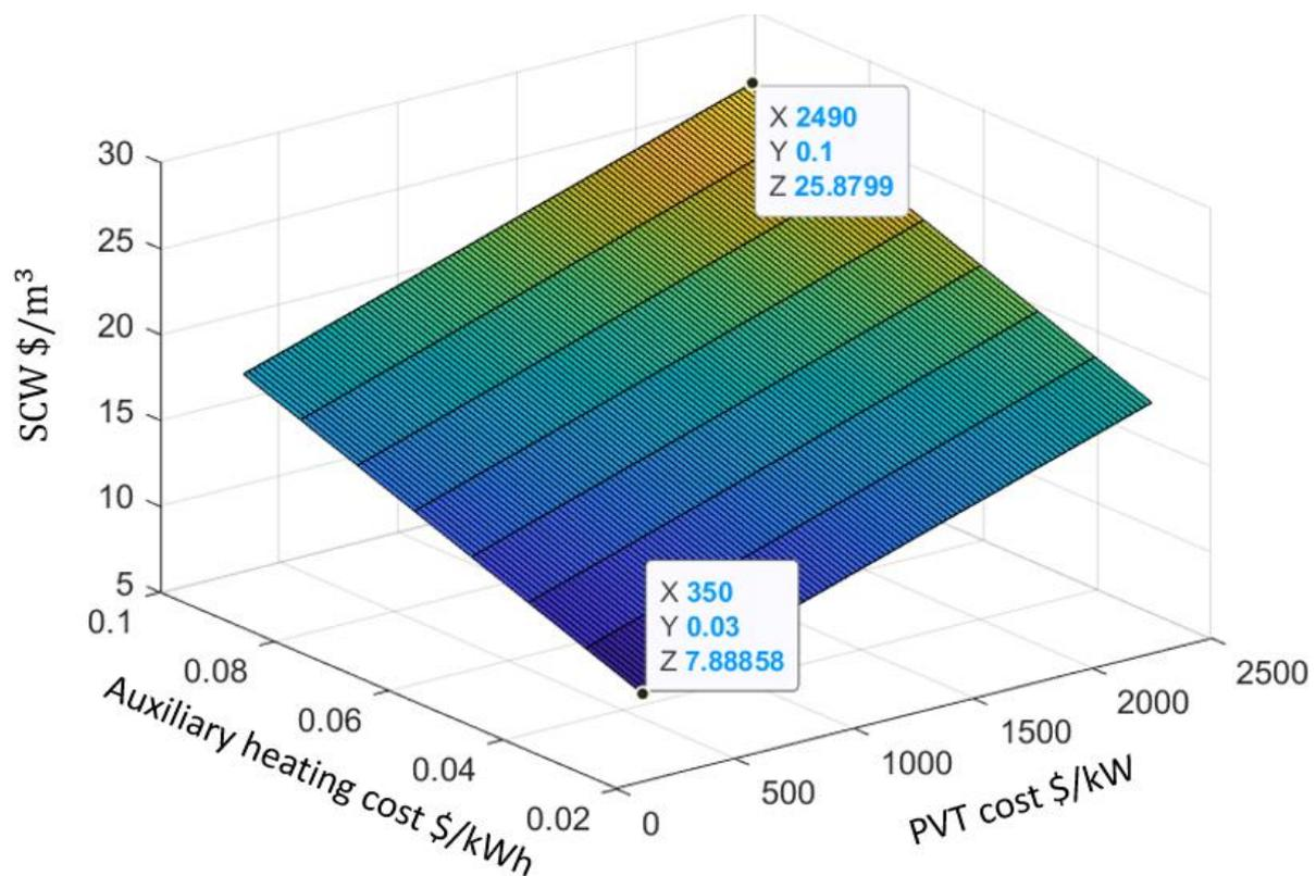
**Figure 13.** The sensitivity of varying PVT capital and installation cost and the required auxiliary heating on the SCW.
