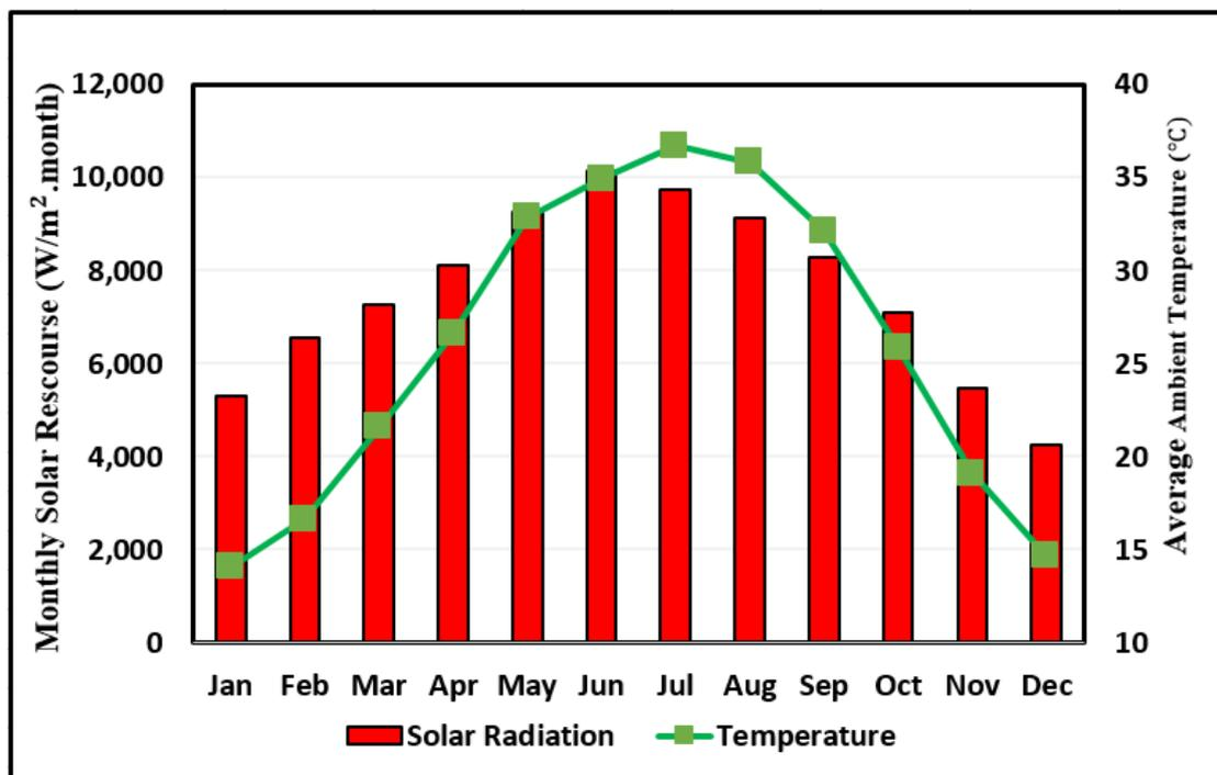
**Figure 6.** Weather condition for the selected location showing Global horizontal irradiance vs. ambient temperature.
