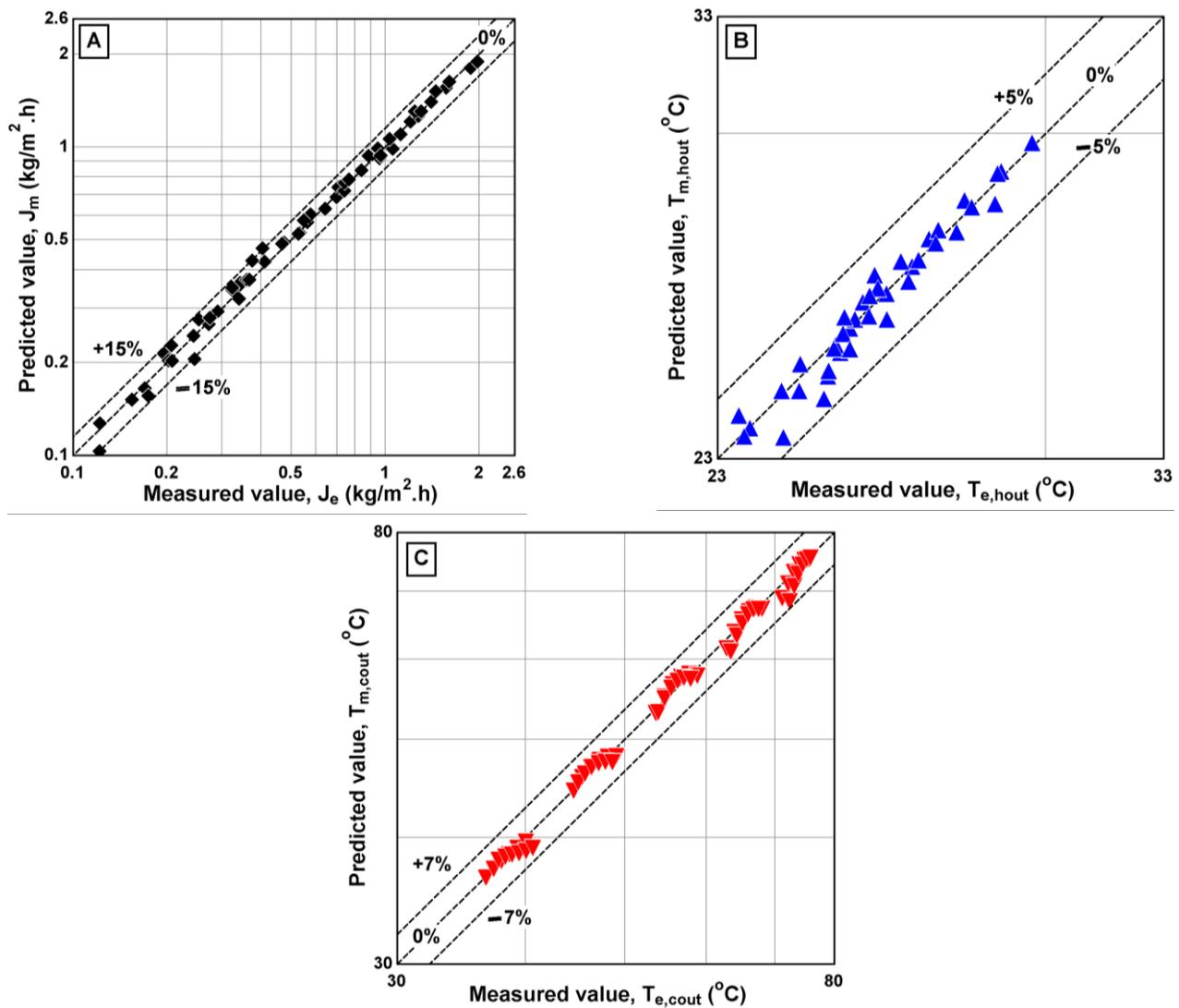
**Figure 4.** Comparison between experimental and model results of the DCMD module (A) Permeate mass flux, (B) Outlet of hot water temperatures, and (C) Outlet of cold-water temperatures.
