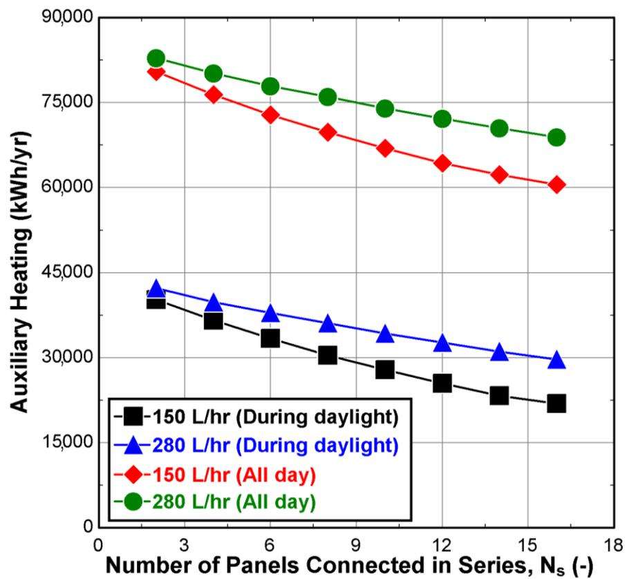
Figure 9. Annual auxiliary heating as function of number of panels and mass flow rate.
