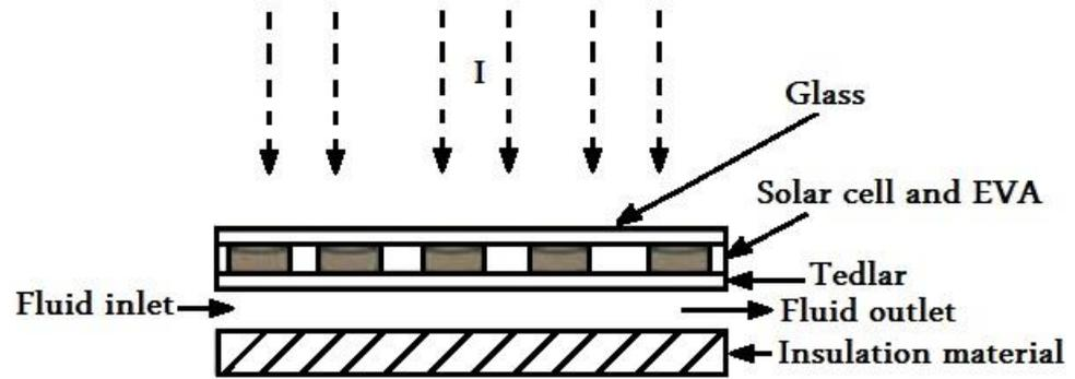
Figure 3. Block diagram for the PVT [28].
