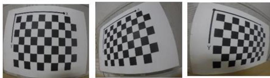
Figure 5. Example images of a checkerboard calibration patterns.
