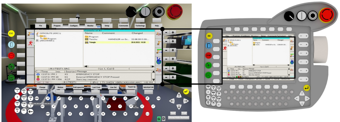
Figure 10. The user interface of the digital twin compared to the teach pendant.
