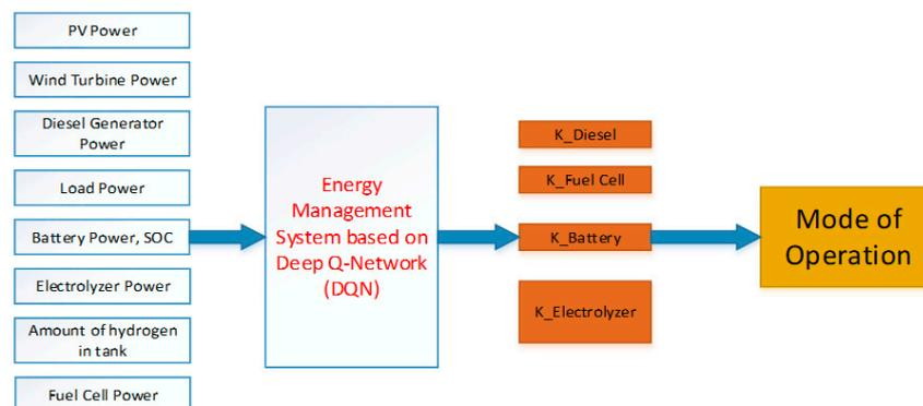
Figure 2. The proposed Deep-Q-Network-based EMS.
