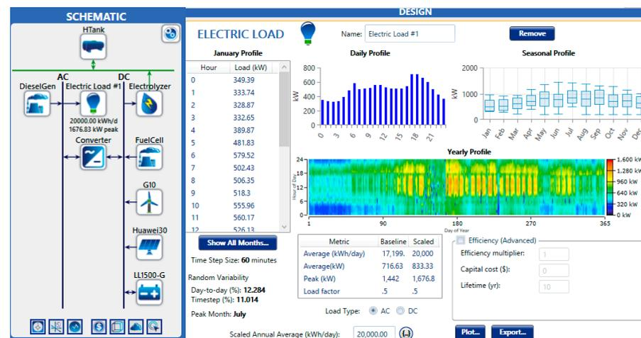
**Figure 7.** The proposed HRES (left) and the load demand at Basco station (right) presented in HOMER software.
