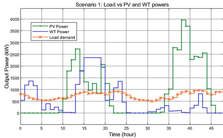
Figure 10. Load demand, PV, and WT power in Scenario 1.
