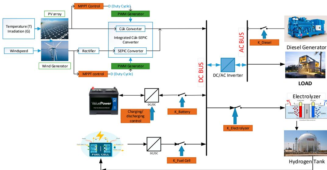
Figure 1. The diagram of the proposed HRES.
