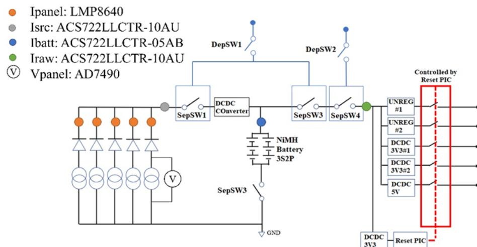
Figure 3. EPS block diagram with power distribution.
