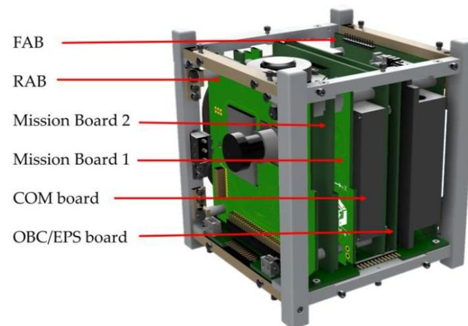
**Figure 1.** Bus system configuration.
