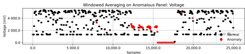
Figure 9. Initial voltage data plot after windowed averaging.
